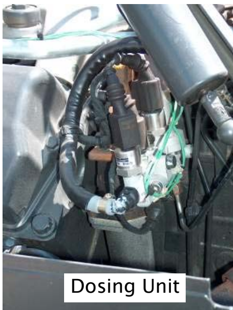
Figure 16: Dosing Unit, Urea Solution Injection Nozzle
