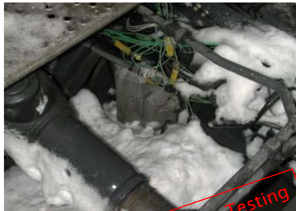
Figure 12: AdBlue Supply Unit mounted next to AdBlue Tank
