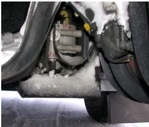
Figure 12: AdBlue Supply Unit mounted next to AdBlue Tank
