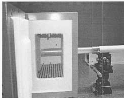
Figure 5.18(b) Sensing head in the high temperature furnace
