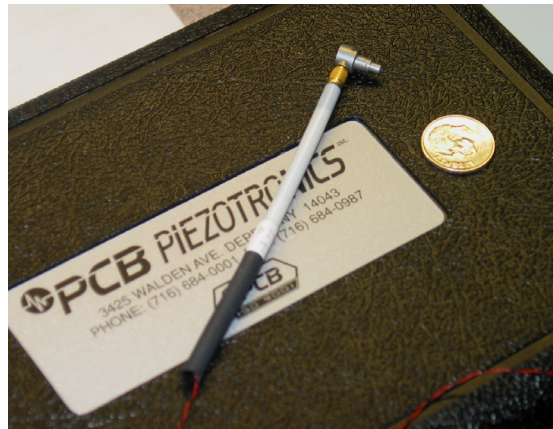
Figure 5: Excitation hammer from PCB piezotronics.
