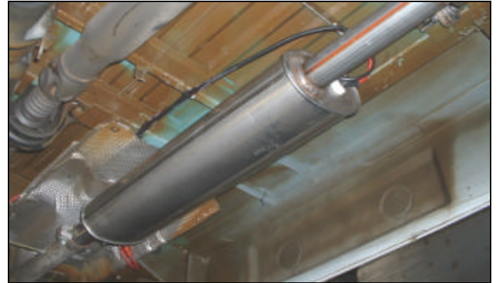
Fig 16 - Installation of PowerTrap Silencer on VW LT35 Van
