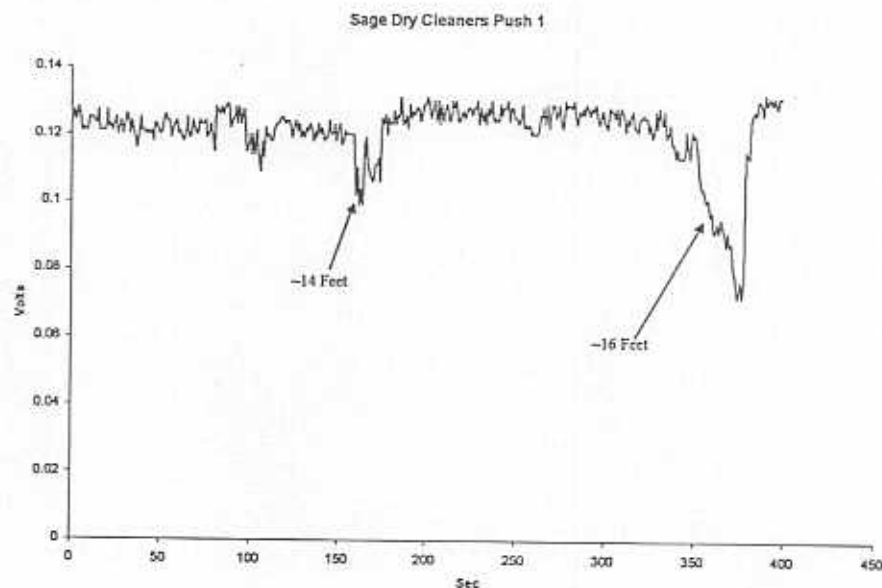
Figure 15. Expanded view of the IRS response in the first push at Sage Dry Cleaners.
