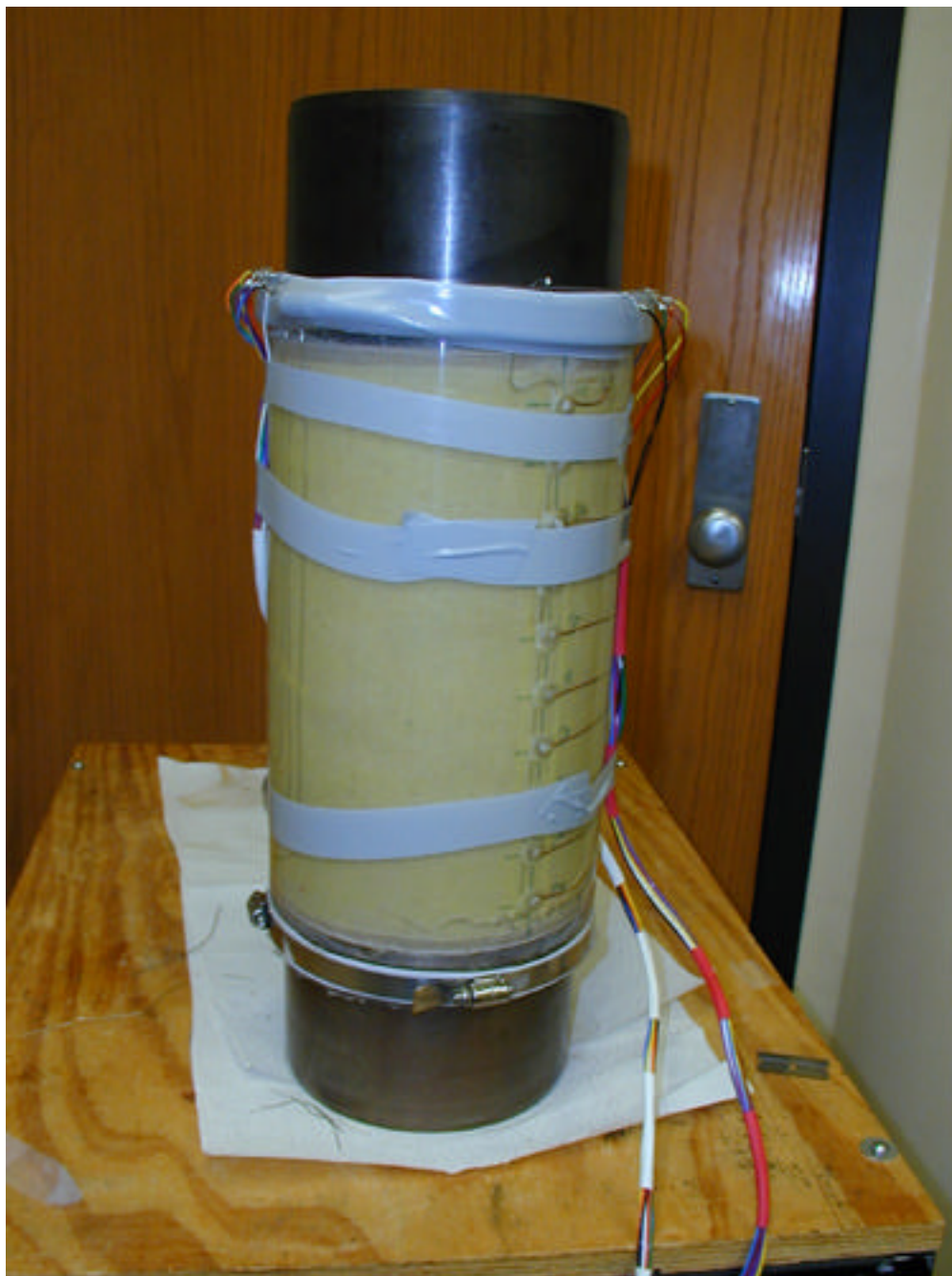
FIG. 73. A photograph of the jacket/sample assembly for vertical tomography.
