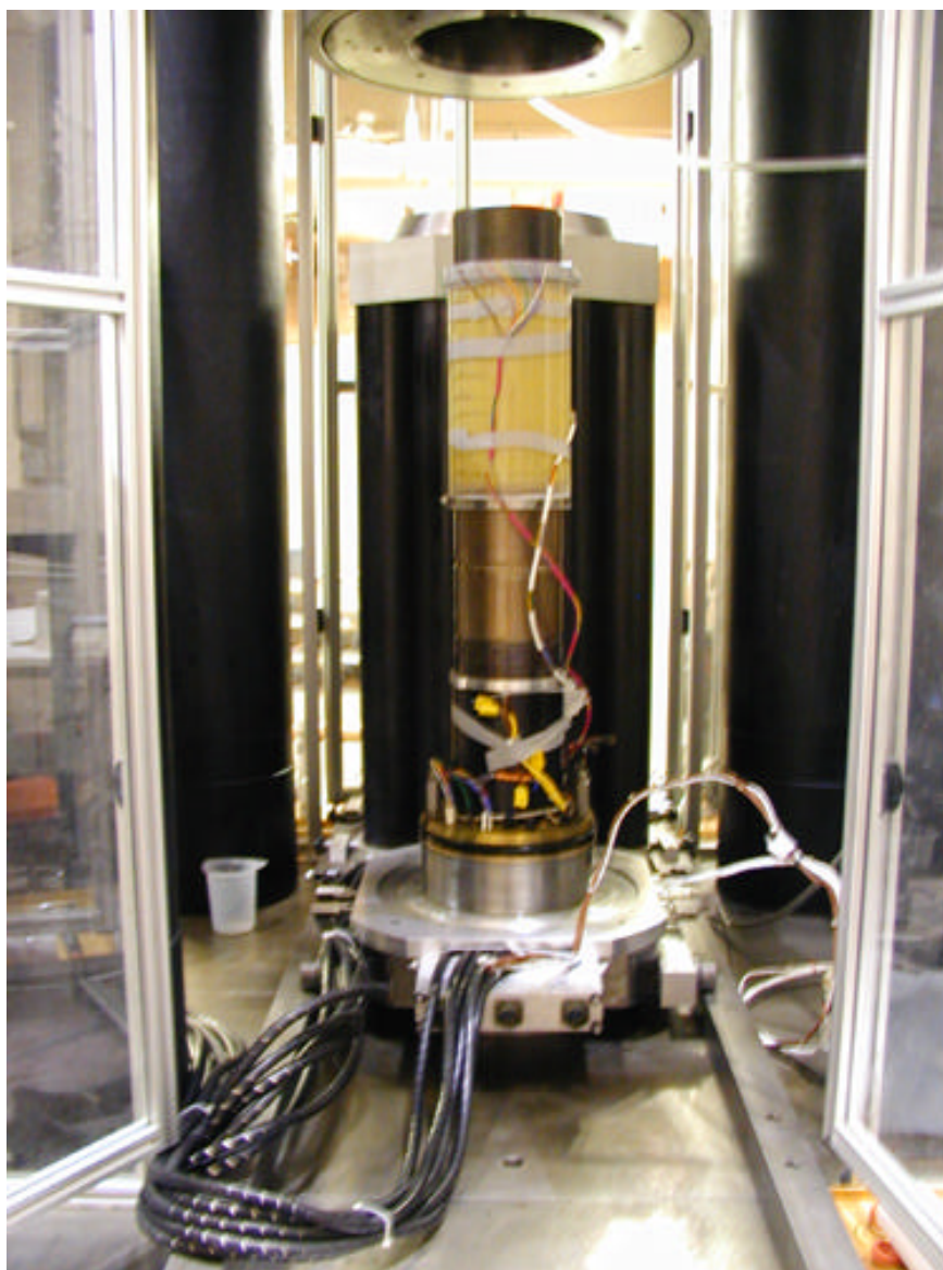
FIG. 74. A photograph of the sample in the Keck load frame before insertion into the pressure cell
