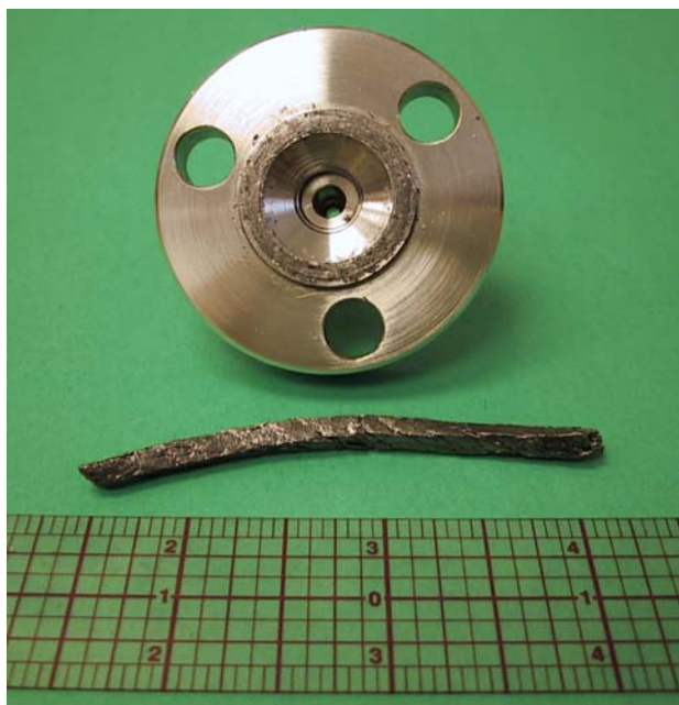
Figure 1. 25 mm Millipore membrane cell with high temperature Grafoil valve packing material used in place of a polymer o-ring. Maximum use temperature of Grafoil material is 650°C.
