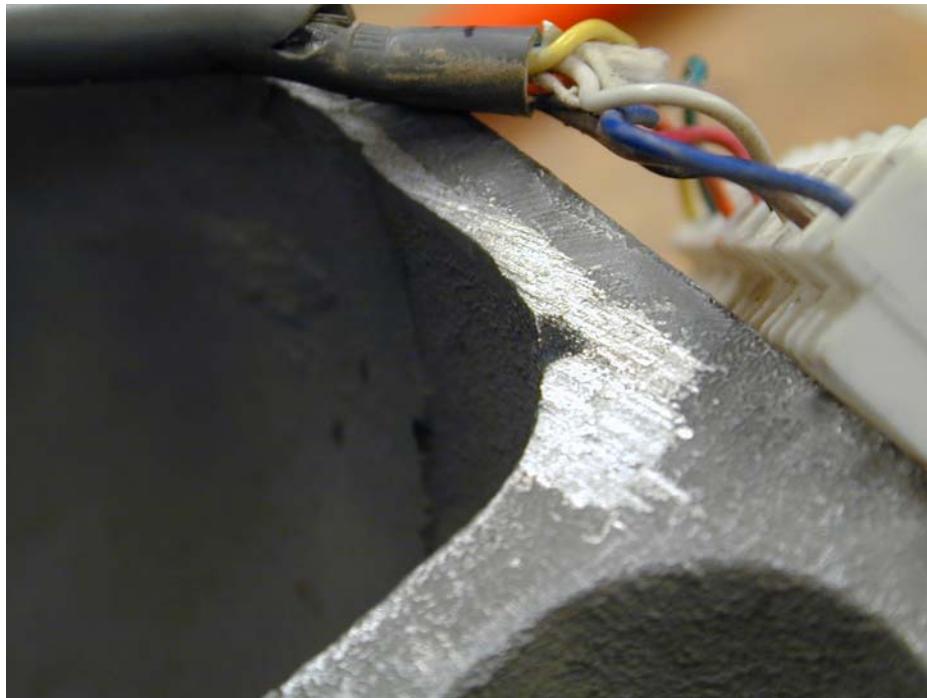
Photo 5. One more location where the two turbine body halves were rubbing, again on the generator portion.
