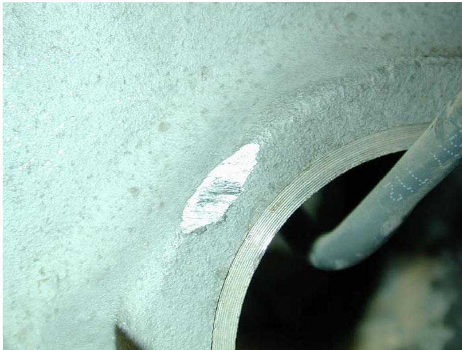
Photo 3. There were a few locations where the upper body (furling generator portion) was rubbing the lower turbine body. Here we can see some rubbing on the generator portion.
