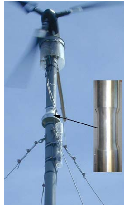
Figure 4. The tower bending transducer was custom-built to allow for higher strain, resulting in a measurable signal even during lower wind speeds.
