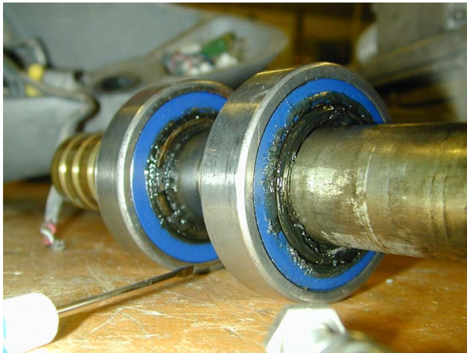
Photo 7. The yaw bearings rotated smoothly and did not show any significant signs of wear but were greasy on the outside. The presence of grease indicates that the seals were starting to fail.
