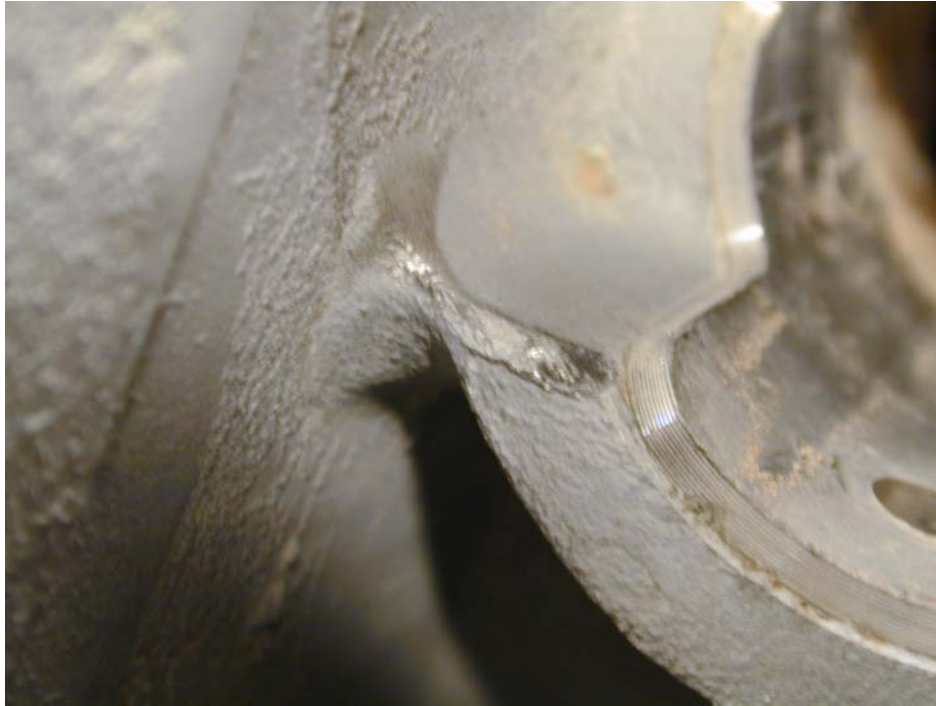
Photo 4. Another location where the two turbine body halves were rubbing, this on the generator portion.
