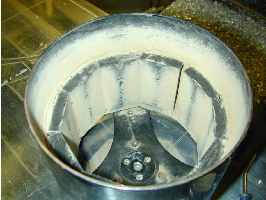
Photo 2. Minor wear can be seen on the magnets where they were in contact with the generator laminates.
