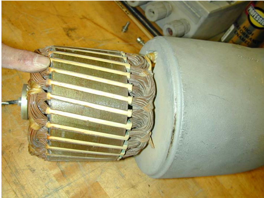
Photo 1. Some wear was seen where the magnet can was rubbing the main turbine housing.
