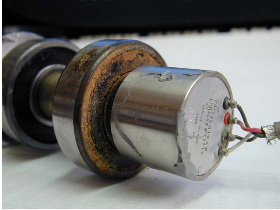
Photo 8. The rotor bearings rotated smoothly and did not show any significant signs of wear. The inner bearing (furthest from the rotor) was rusty indicating that moisture was trapped and made this bearing very difficult to remove. Note that the slipring shown in the photo is not standard. It was used to power a telemetry transmitter for blade load measurements.
