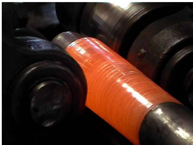
Figure 1. Helical cross rolling of MA956 tubes at 900°C
