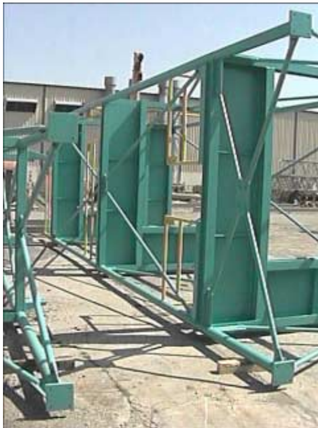
Figure 10: Advanced ElectroCore Module Support Frame After Painting
