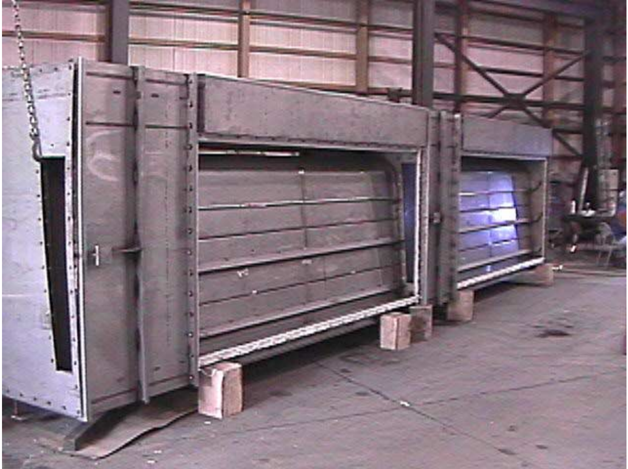
Figure 8: Partially Assembled Advanced ElectroCore Module
