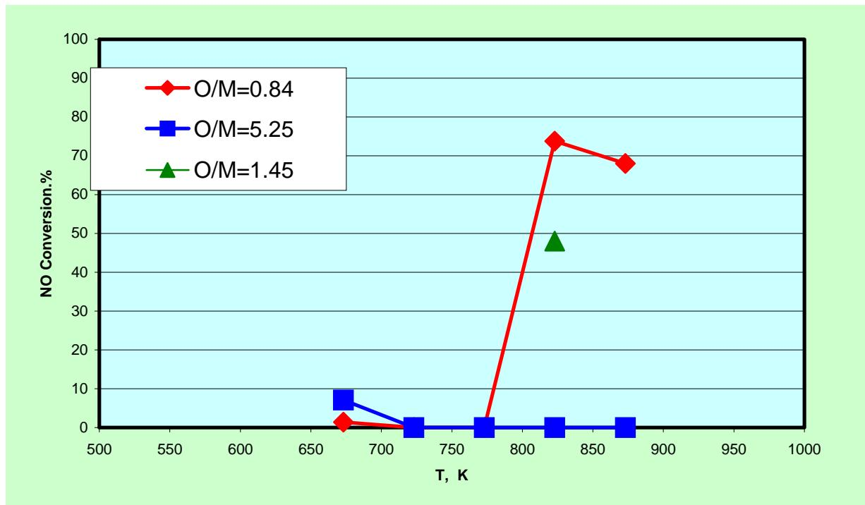
FIGURE 3. NO Conversion by  $\text{CH}_4$  on sulfated catalyst  $\text{Cu}_2\text{Ce}_6$  in the presence of oxygen, wet,  $(\text{O}_2/\text{CH}_4=5.25)$
