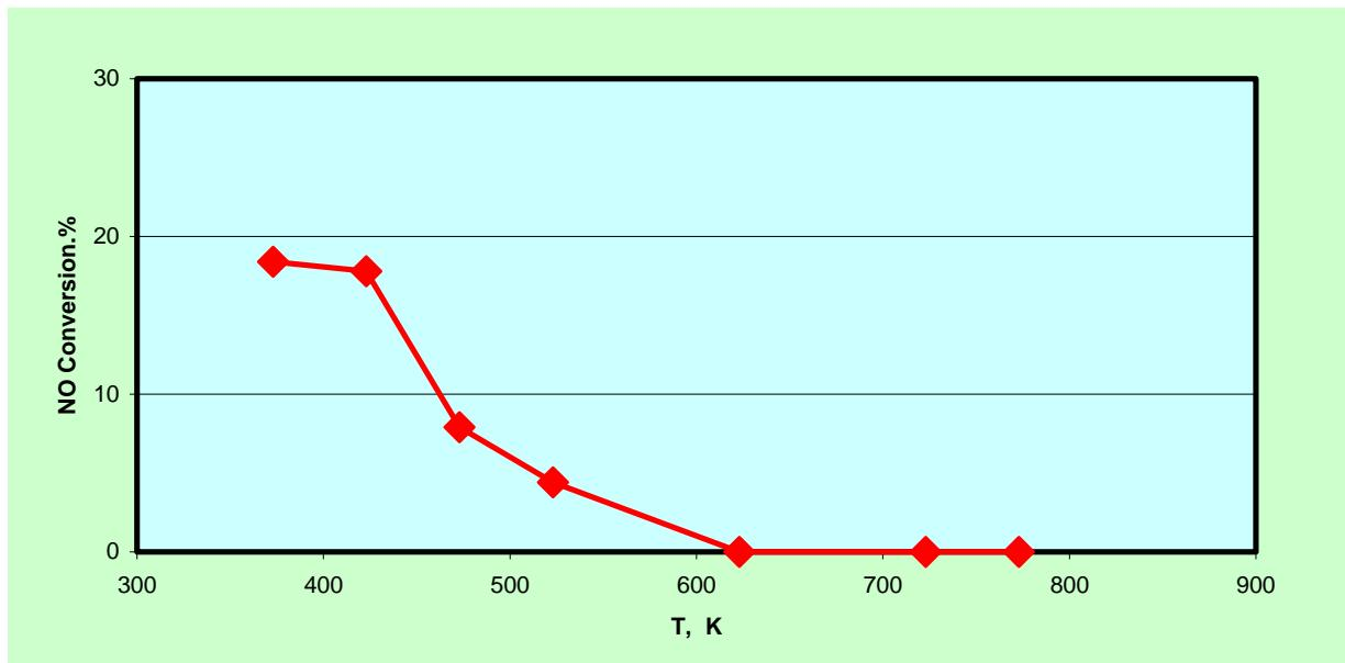
FIGURE 4. NO Conversion by  $C_3H_6$ , Cu8Ce2 catalyst, wet, NO/P=1
