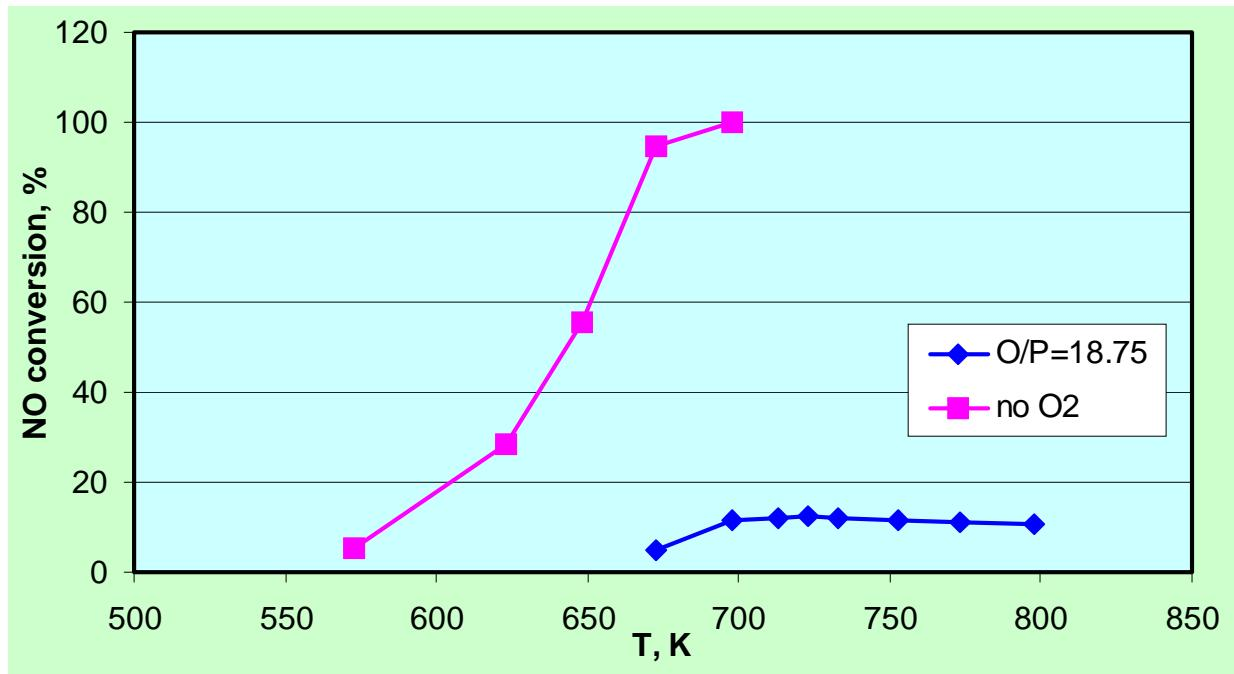
FIGURE 5. NO Conversion by  $\text{C}_3\text{H}_6$ ,  $\text{Cu}_2\text{Ce}_6$  catalyst, wet,  $\text{NO}/\text{P}=1$
