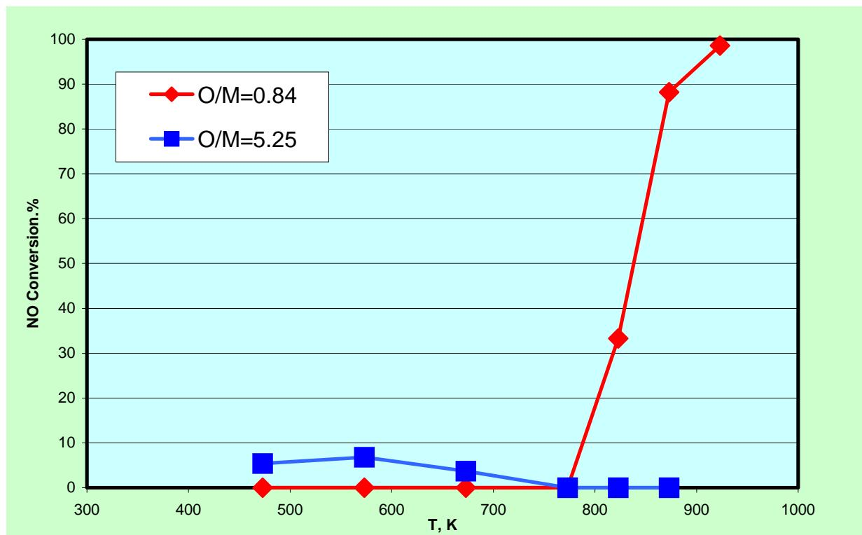
FIGURE 2. NO Conversion by  $\text{CH}_4$  on catalyst Cu7.5Ce2.5 in the presence of oxygen, wet
