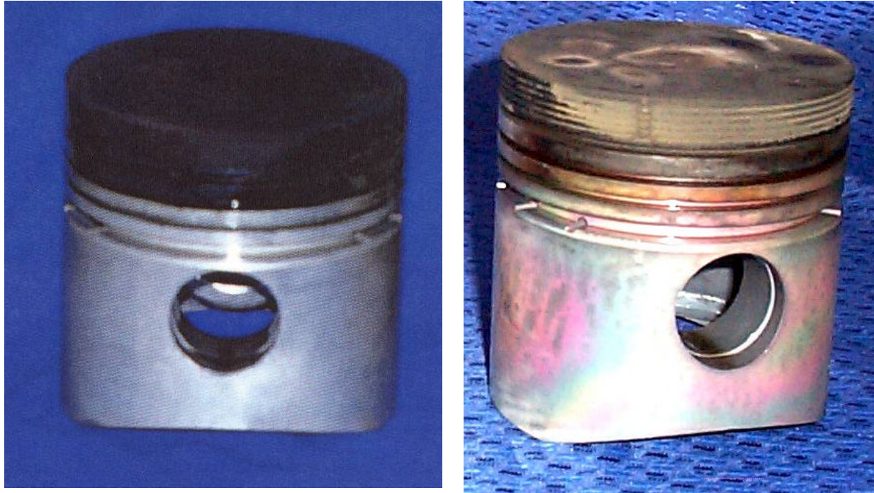
Fig.9. Comparison of Uncoated and Coated Pistons from Yanmar Single Cylinder Diesel Engine Tests. Test Conditions Include: Steady Speed @ 2200 RPM, Full-Load, Test Time – 50 Hrs Fuel – No. 2 (39 ppm S), Lube Oil – 10W30
