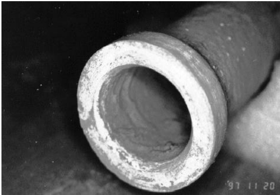
Figure 48 - Inside diameter of Karhula-exposed element before ash removal
