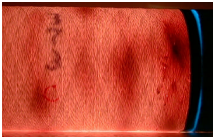
Figure 32 - ID P.I.T. evaluation of original “hoop-only dual membrane” filter (1995)
