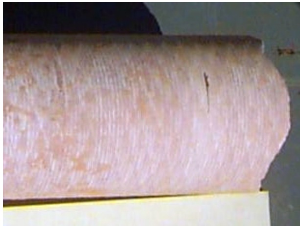
Figure 82 - Broken end of Filter C752, with deep chip 1 1/4" below the break
