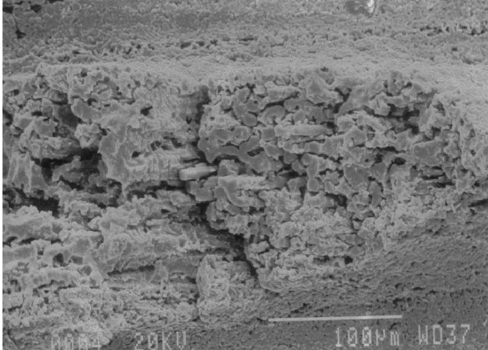
Figure 61 - UNEXPOSED CANDLE, individual “yarn bundle” (300X)
