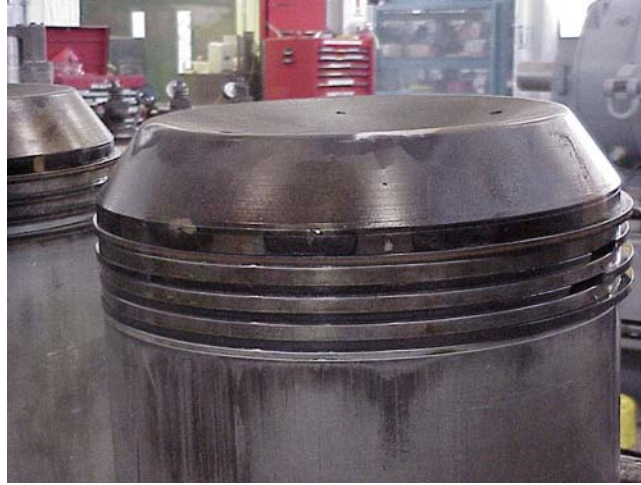
Figure A20-17: Cylinder 1 Modified Piston - Pilot Fuel Injector
