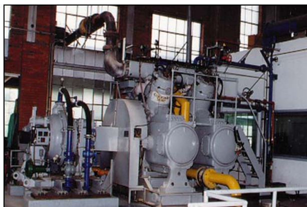
Figure A16-1: The Cooper Bessemer GMV-4TF Large Bore Natural Gas Engine.
