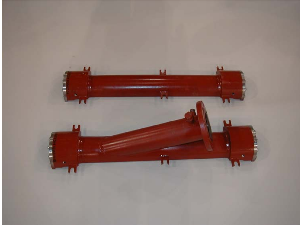
Figure 21. Cast Iron Entry Fitting (4-inch Prototype)
