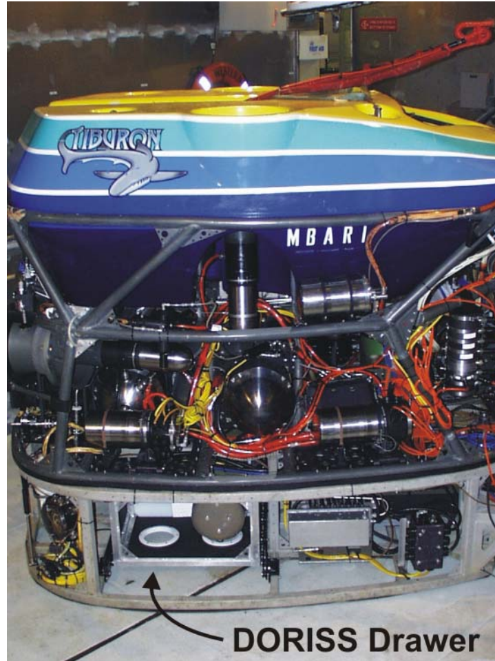
Figure 1. MBARI's remotely operated vehicle "Tiburon", in side view. The base vehicle weight is 3,084 kg. Front, with manipulators and cameras not shown, is to the right of the image. The syntactic foam pack that provides buoyancy is on top, the core vehicle power, thrust, telemetry, and computing, systems are housed in the middle. Below is the tool sled with the drawer used to house the Deep Ocean Raman In-Situ Spectrometer (DORISS) system seen at bottom left.
