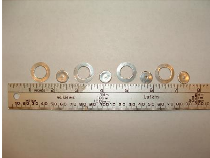
Figure 3: Bluff body structures for Reactor A
