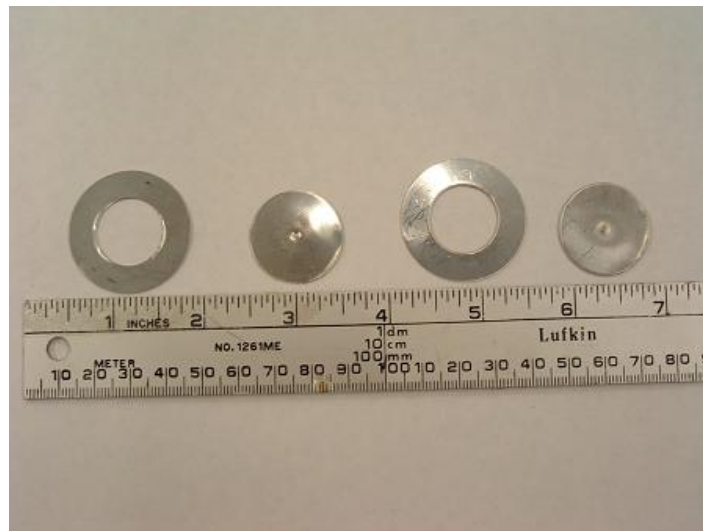
Figure 4: Bluff body structures for Reactor B
