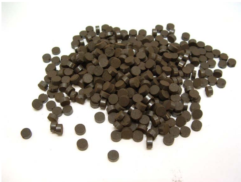
Figure 66: Sud Chemie pelletized FCRM-2 catalyst
