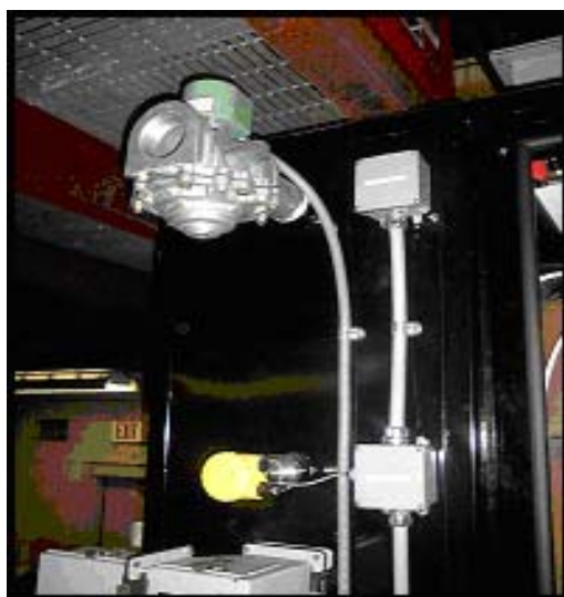
Figure 67 Pressure and oxygen sensors were used to monitoring the chamber pressure and oxygen concentration in the separation chamber.
