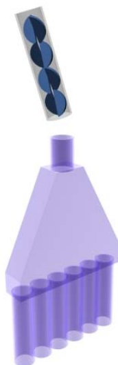
Figure 18 Bench-scale tribocharger made of Plexiglas used in conjunction with the drum-type bench-scale triboelectrostatic unit.
