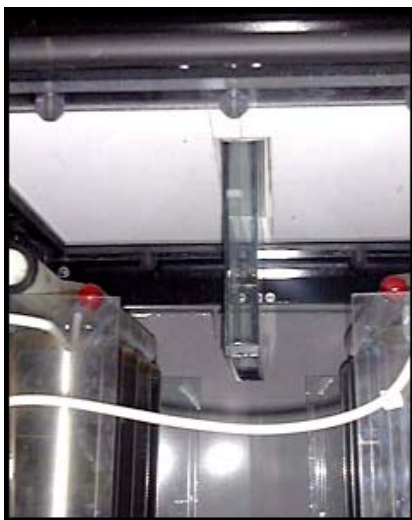
Figure 63 Feed introducer made of tempered glass was used to direct the feed material into the separator chamber.
