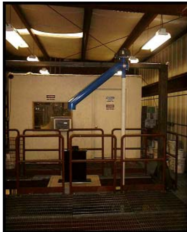
Figure 62:POC Scale tribocharger made of copper used for the preliminary separator study.
