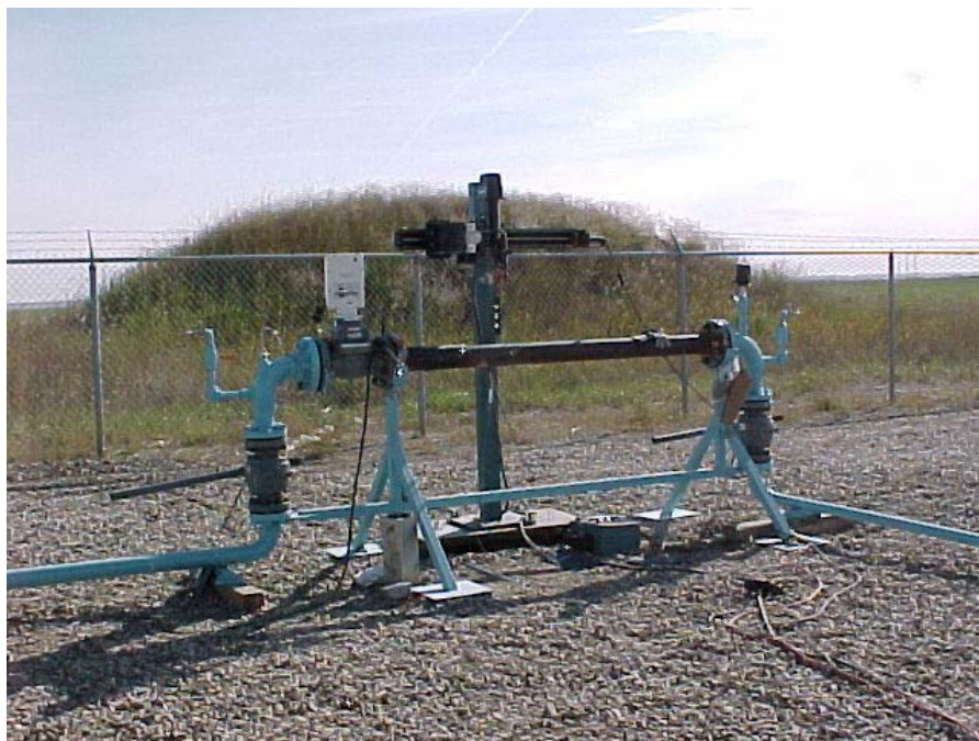
Figure 15 - Experimental Set-Up for Welding onto Thin-Wall Pipe containing Pressurized Methane Gas
