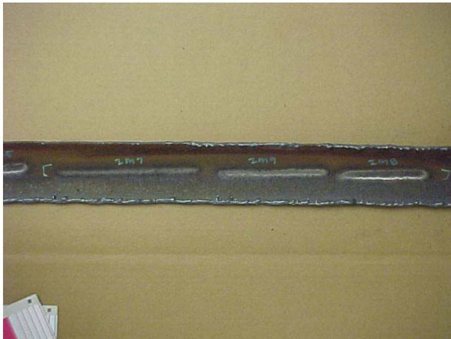
Figure 17 - Internal Appearance of Welds Shown in Figure 16
