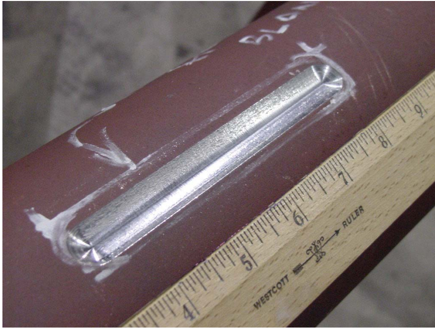
Figure 12 - Long, Shallow Simulated Corrosion Damage
