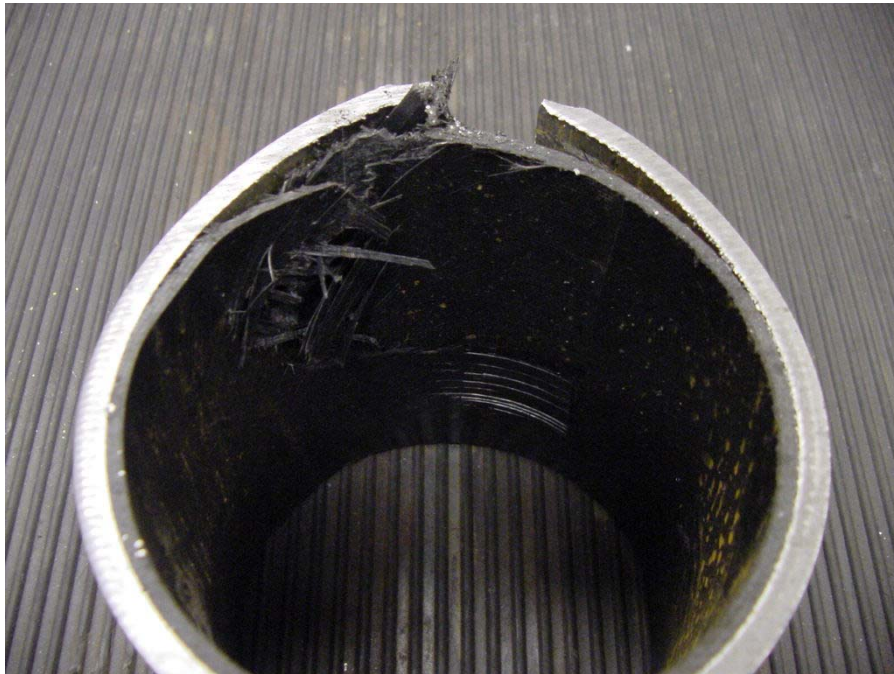
Figure 24 - Fiber-Reinforced Composite Liner in Ruptured Pipe Section Containing Long, Shallow Simulated Corrosion Damage Fiber-Reinforced Composite Repairs
