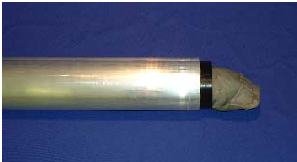
Figure 9 - Silicon Rubber Bag Inserted into Liner
