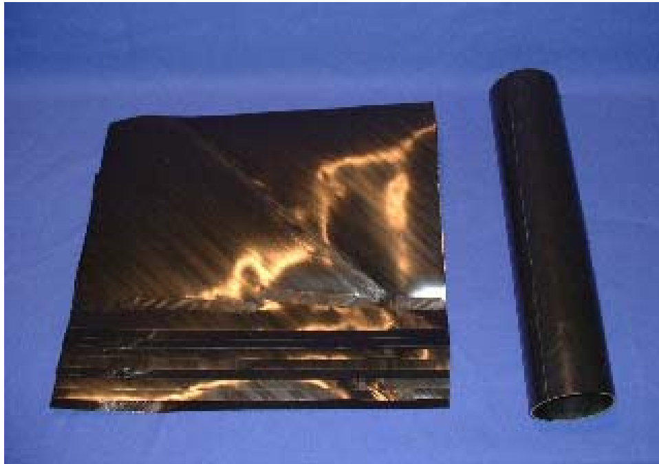
Figure 7 - Lay-Up and Forming of Fiber-Reinforced Composite Liner
