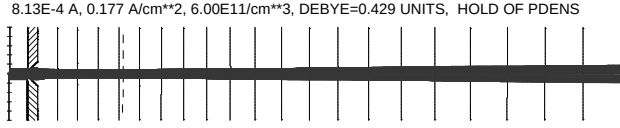
Figure 5. Ion beam dynamics simulation using IGUN. The extractor aperture is 1 mm in diameter and the gap is 63 mm in length. Each of the 24 beam-lets are carrying \sim 0.8 mA of ion current.
