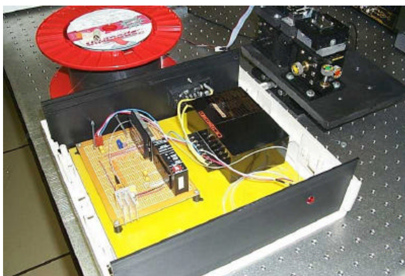
Figure 3.8. Picture of the single-mode white light air gap monitoring system
