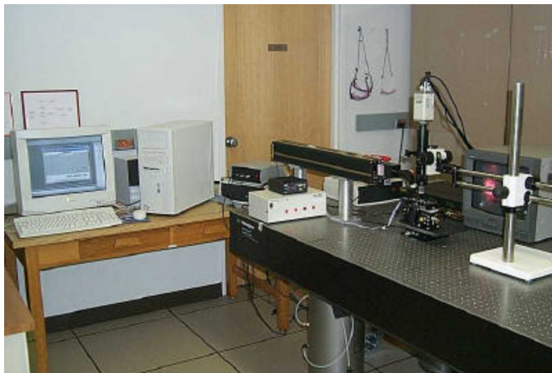
Figure 3.2. Picture of the automated SCIIB sensor fabrication system
