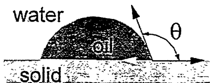
Figure 2. Contact angle is the angle between the tangent to the droplet at the three-phase line and the solid surface, measured here through the water phase.
