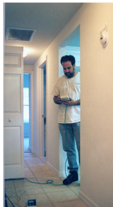
Figure 6 Measuring pressure differentials with digital manometers (circled) during validation exercises in North Florida.
