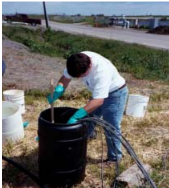
Image 6-3. Pressure transducers were tested for accuracy by submerging the sensors in water at various depths.
