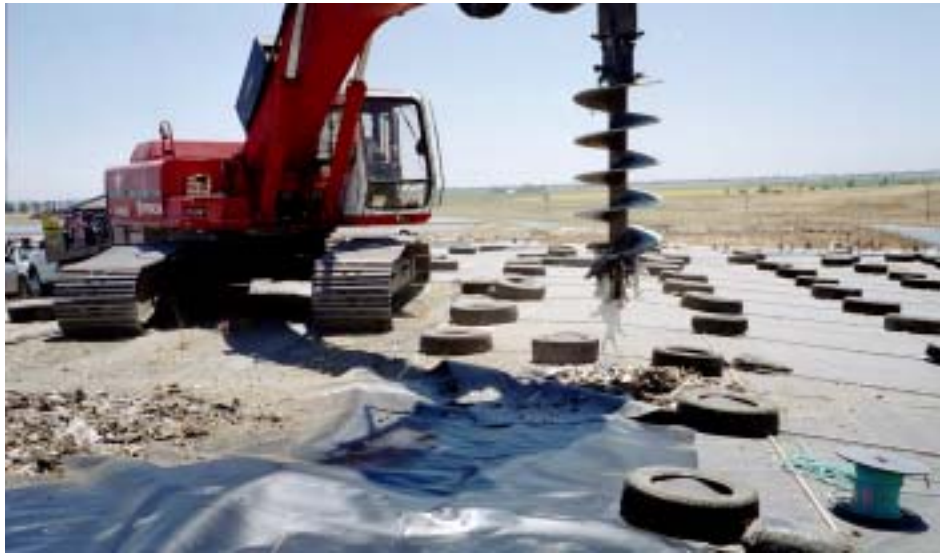
Image 3-9. An excavator-mounted drill rig was used for the sampling event to drill boreholes 25 to 40 feet deep.
