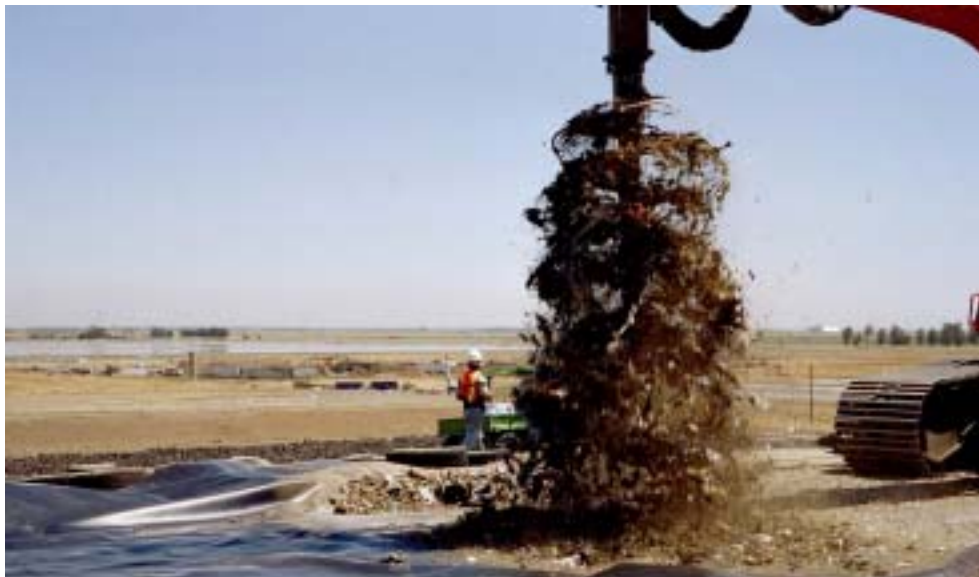
Image 3-10. Excavated waste was placed on liner material located adjacent to the boreholes where samples were then collected.
