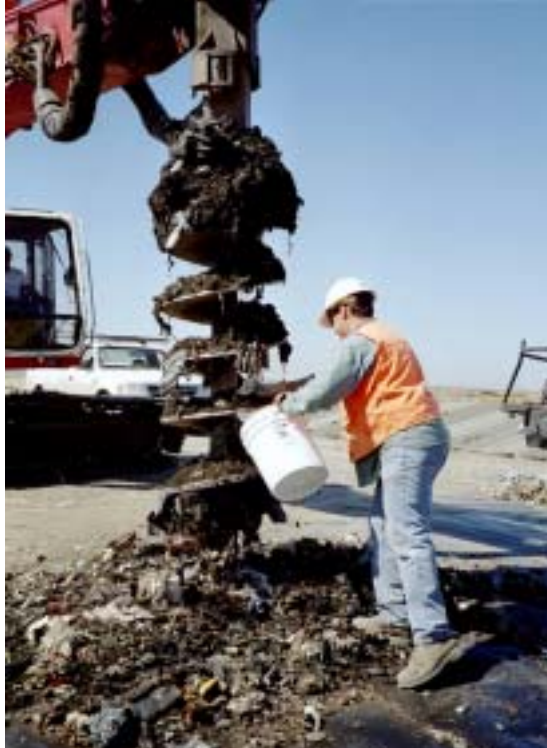
Image 3-11. At select locations, samples were collected directly from the auger to record the temperature of the waste as it was removed from the cell.
