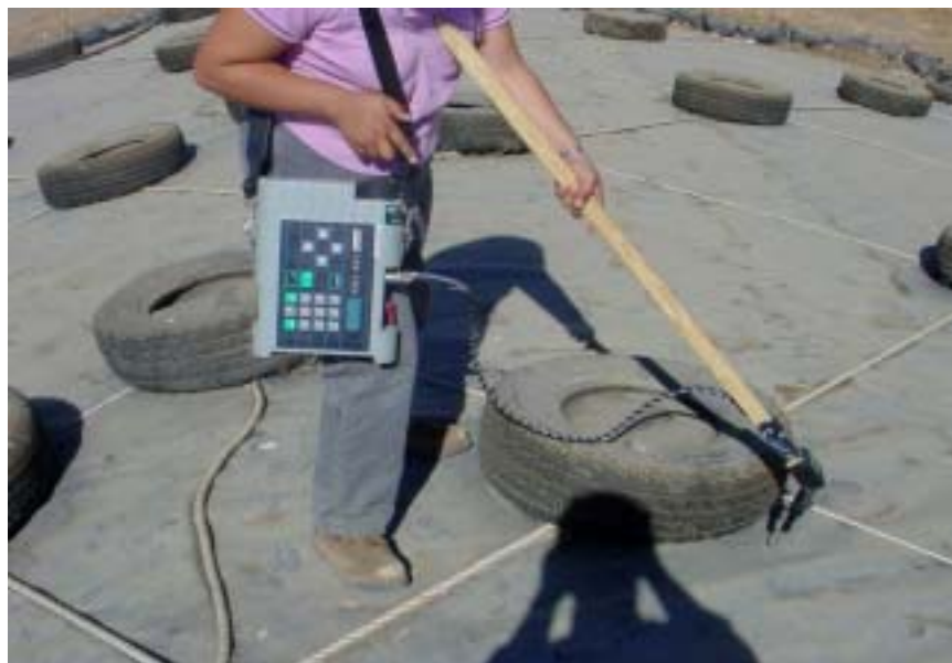
Image 3-6. Surface emission monitoring with the TVA 1000.
