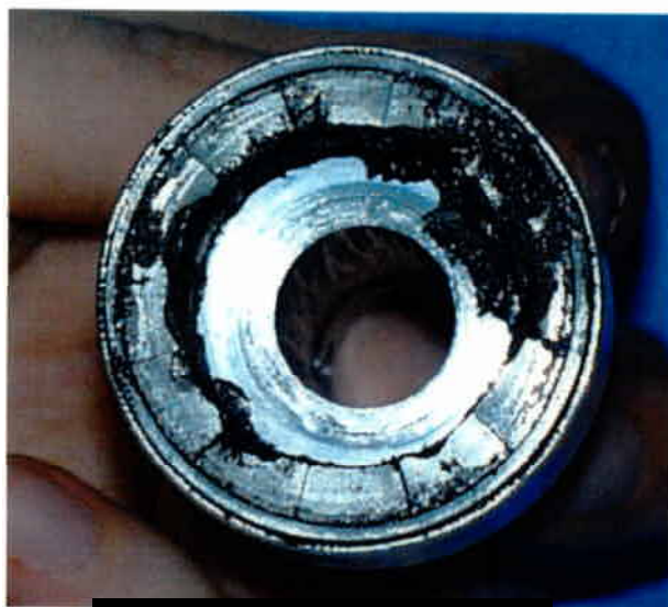
Figure 16. Damaged magnetic coupling from Tuthill gear pump.
