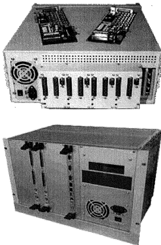
Fig. 1. PCI (top) and cPCI (bottom) data acquisition systems. (Images printed with permission of D-TACQ Solutions Ltd.)
