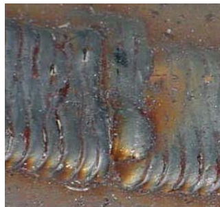
7:00 – Bad Appearance Due Robot Program Error
