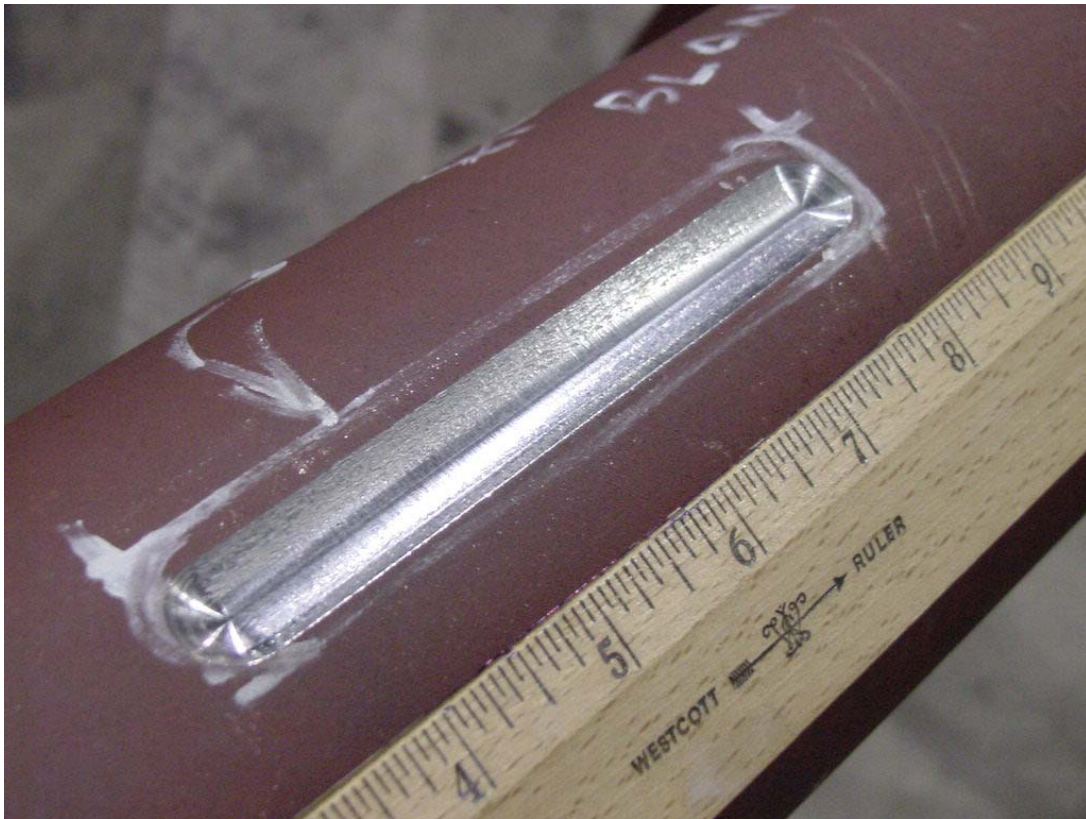
Figure 12 - Long, Shallow Simulated Corrosion Damage
