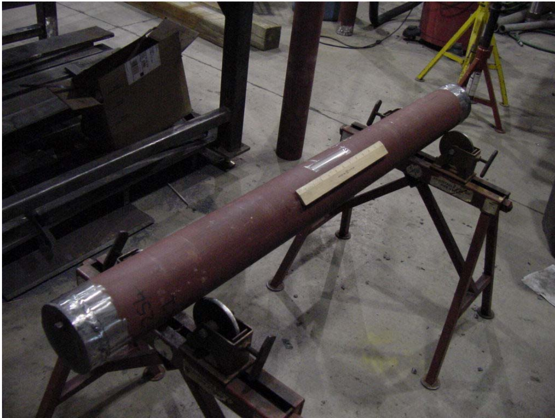
Figure 14 - 114.3 mm (4.5 in.) Diameter Pipe with End Caps Welded and Simulated Corrosion Damage Introduced
