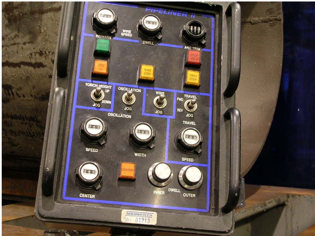
Figure 23 - Magnatech Control Pendant Showing Control Parameters
