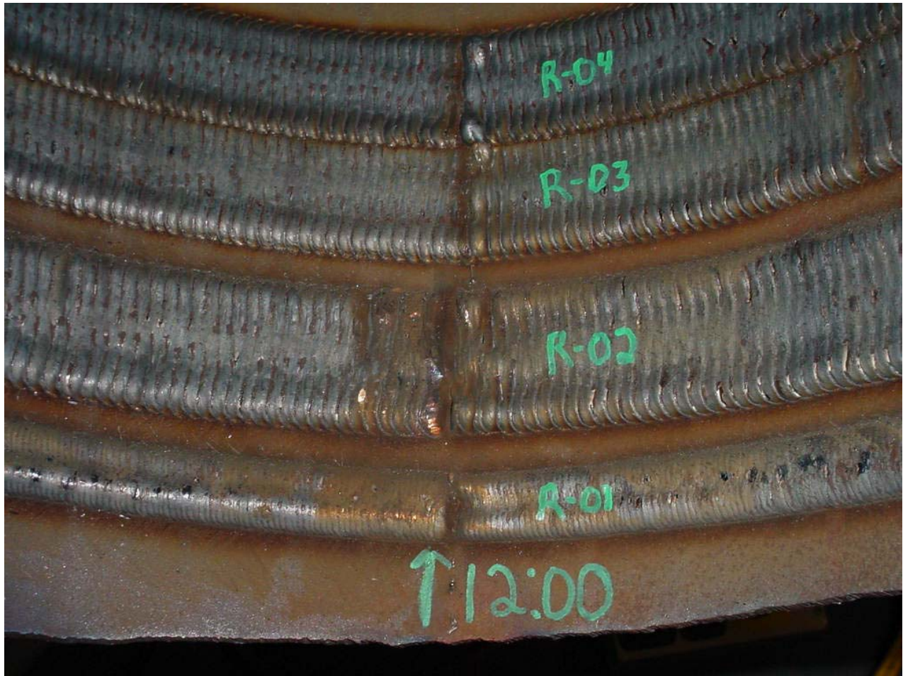
Figure 54 - Tests R-01 through R-04 at 12:00 (Note the Poor Tie-Ins for R-01 through R-03)
