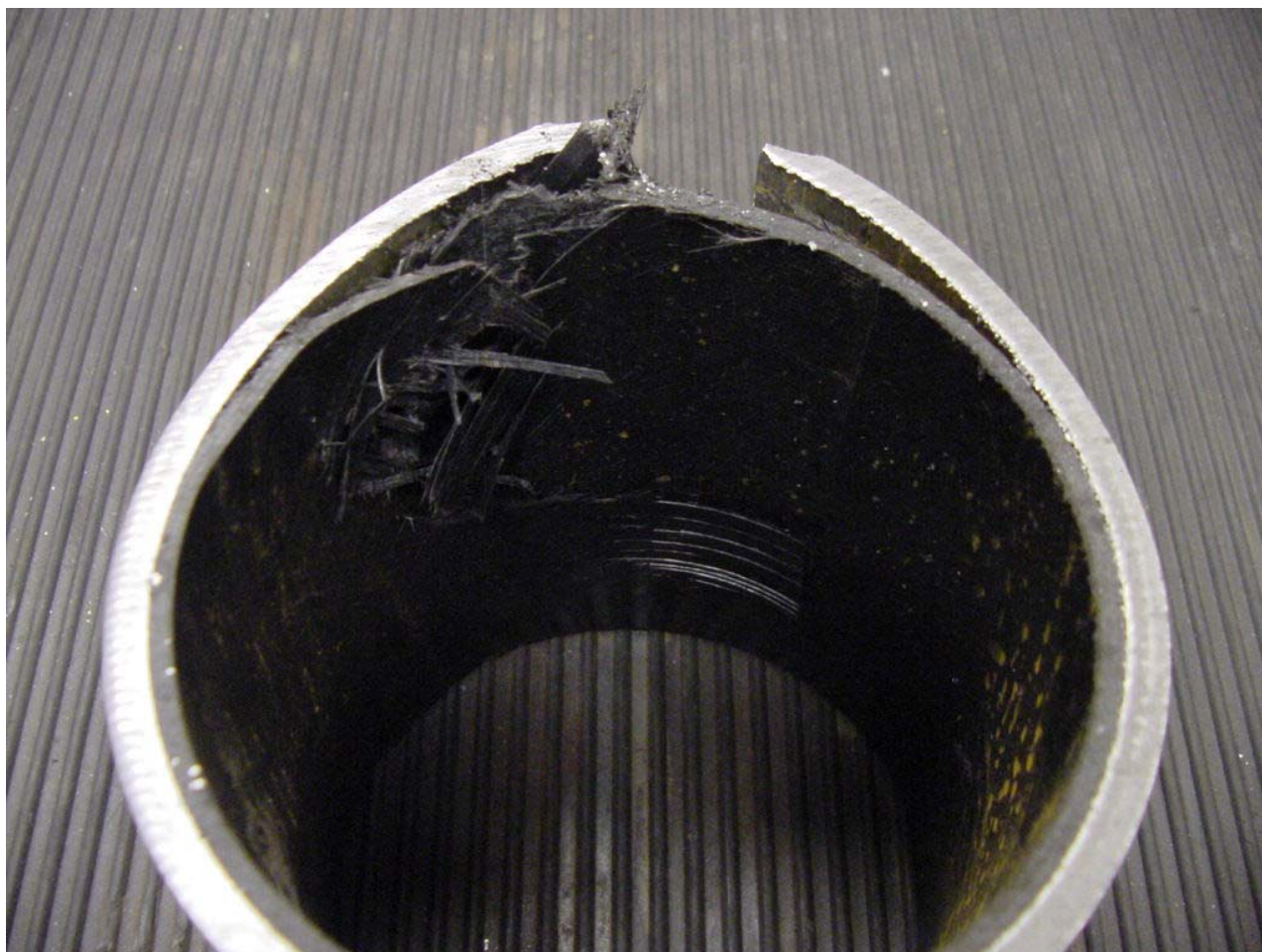
Figure 64 - Pipe Sample Containing Round-Bottom Longitudinal Slot Showing Rupture of Liner Material
