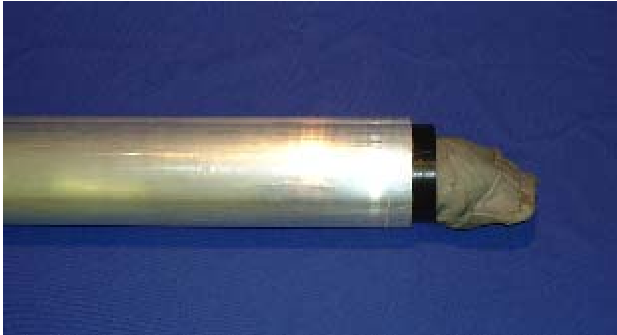
Figure 9 - Silicon Rubber Bag Inserted into Liner
