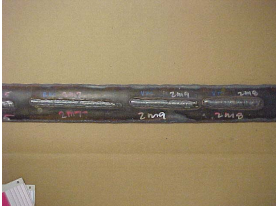
Figure 26 - External Appearance of Welds Made on 3.2 mm (0.125 in.) Thick Pipe with Methane Gas at 4.5 mPa (650 psi) and 6.1 m/sec (19.9 ft/sec) Flow Rate
