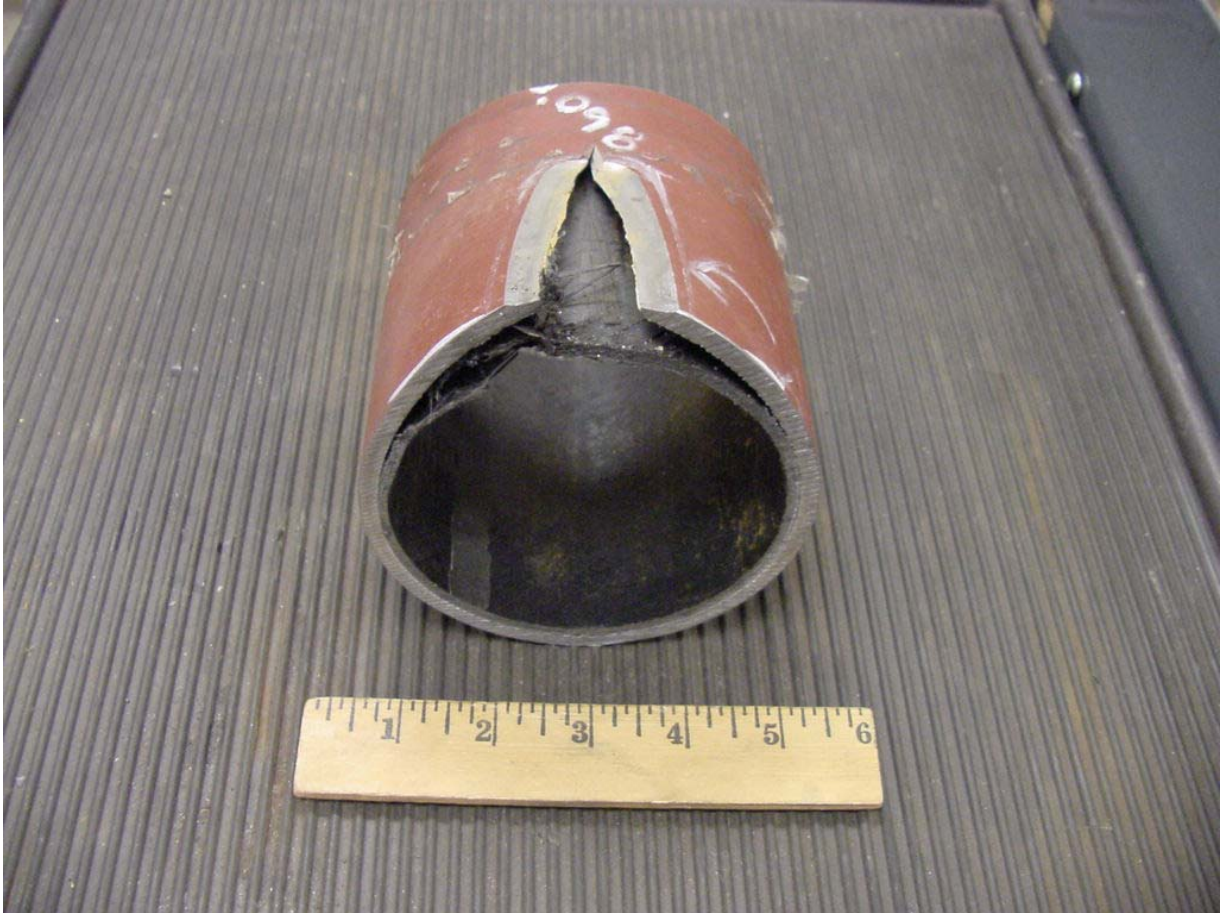
Figure 63 - Water-Jet Cut Section through Pipe Sample Containing Round-Bottom Longitudinal Slot with Liner Installed
