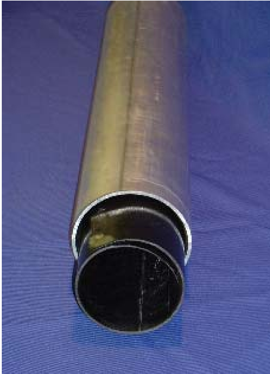
Figure 8 - Insertion of Liner into 114.3 mm (4.5 in.) Diameter Pipe
