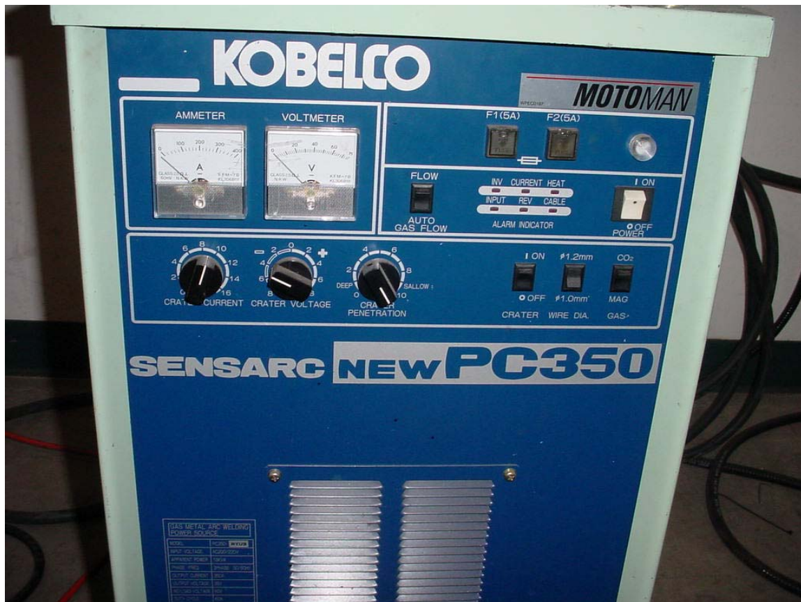
Figure 21 - Kobelco PC-350 Variable Polarity Fuzzy Logic Power Supply
