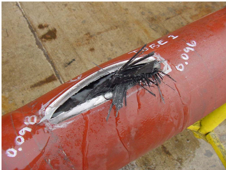
Figure 60 - Pipe Section with Long, Shallow Simulated Corrosion Damage – With Liner – Following Hydrostatic Pressure Test
