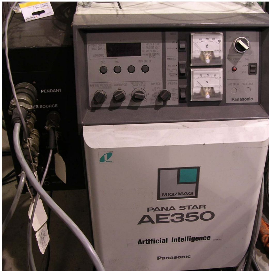
Figure 24 - Panasonic AE 350 Power Supply with Pulse Short-Circuit Metal Transfer Control
