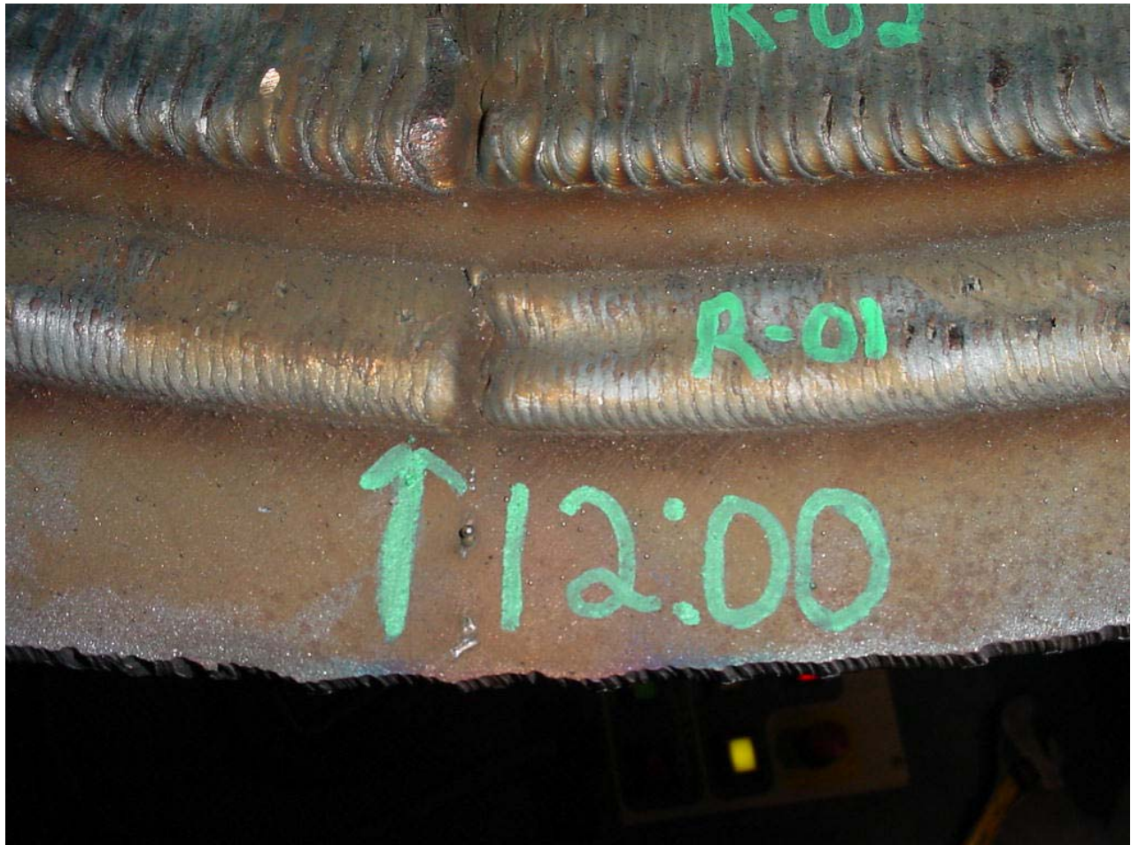
Figure 55 - Test R-01 at 12:00 Showing Poor Stop-Start Tie-In
