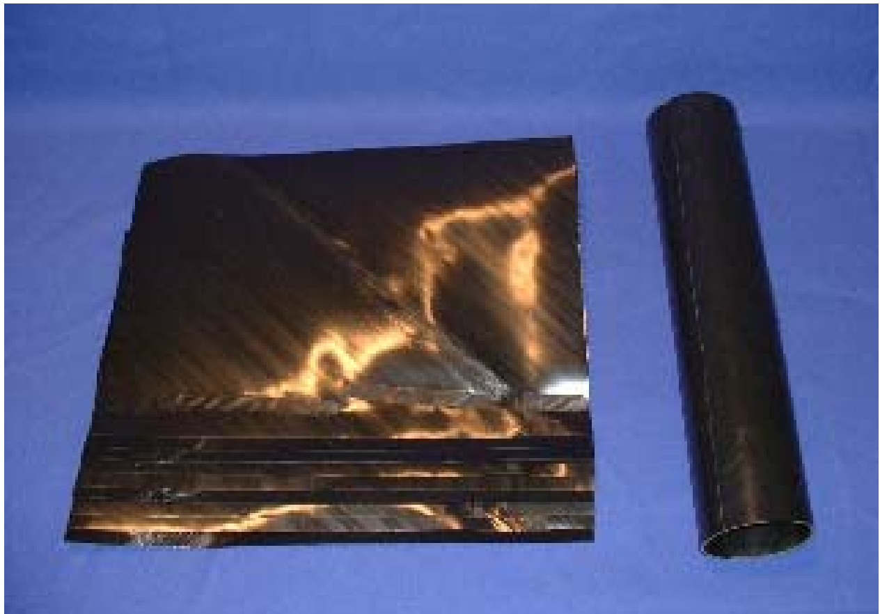
Figure 7 - Lay-Up and Forming of Fiber-Reinforced Composite Liner
