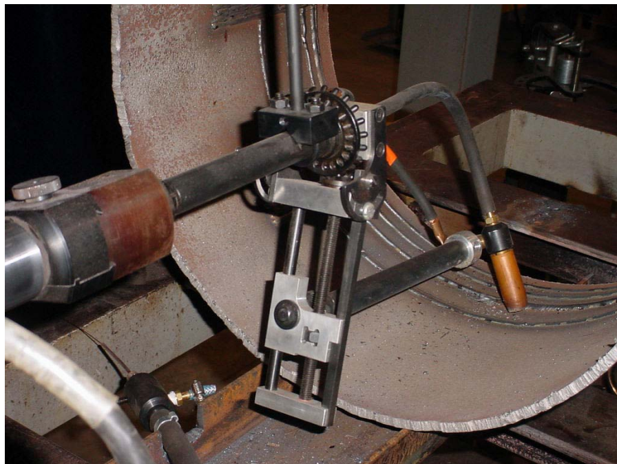
Figure 17 - Bortech Torch and Torch Height Control
