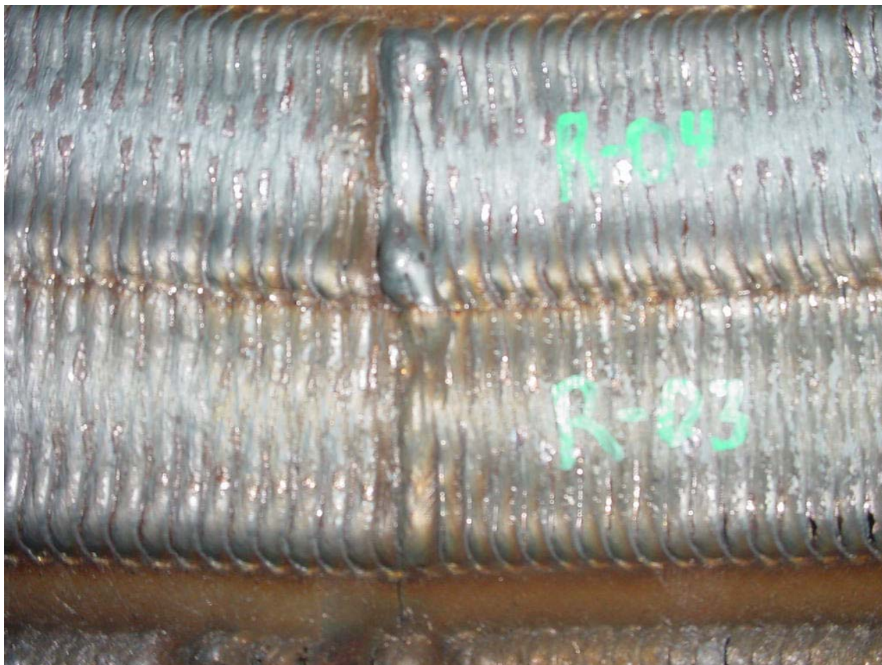
Figure 56 - Tests R-03 and R-04 at 12:00 Showing Better Stop-Start Overlap. (Note that test R-04 was overlapped on test R-03 to provide a larger deposit layer.)
