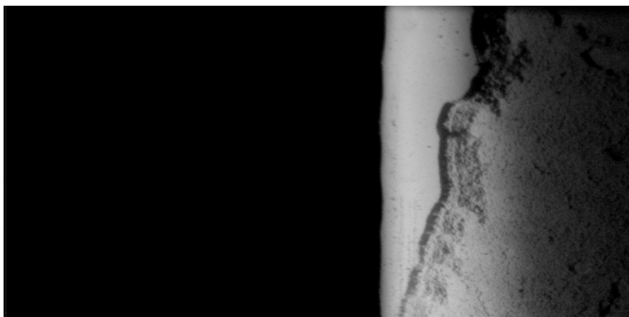
Figure 6.3.20a Effect of face velocity on Lanxide filter Surface quality during long term test cycles 95 psi regeneration pressure, 7 cm/s face velocity , 20 min build-up time. (Contd.)
