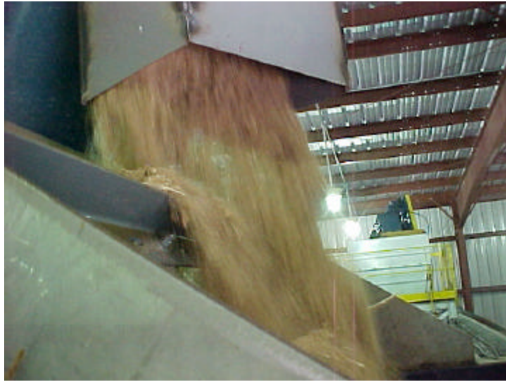
Figure 4. Feeding sawdust to the disc screen at Albright Generating Station
