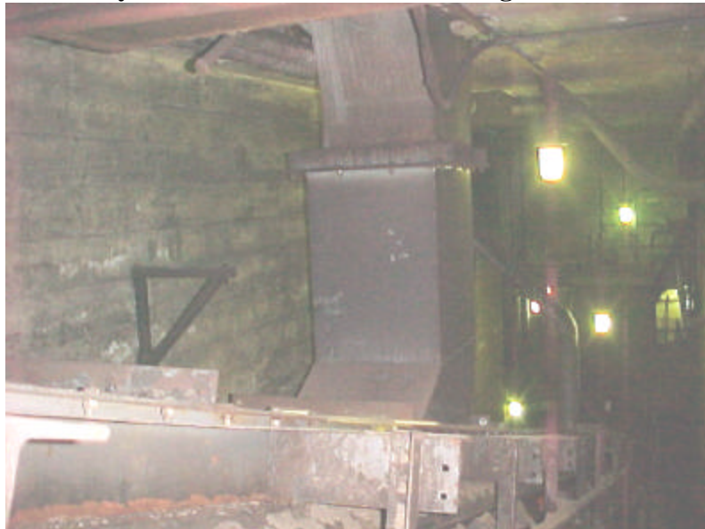
Figure 11. Sawdust discharge chute connecting to the main coal belt.
