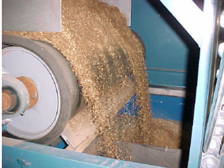
Figure 6. Feeding sawdust to the rotary airlocks at Albright Generating Station
