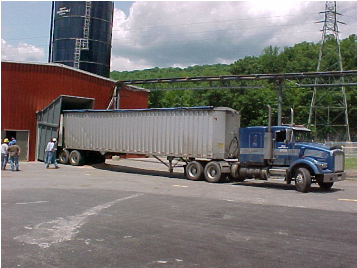
Figure 1. A walking floor van unloading to the walking floor unloader.
