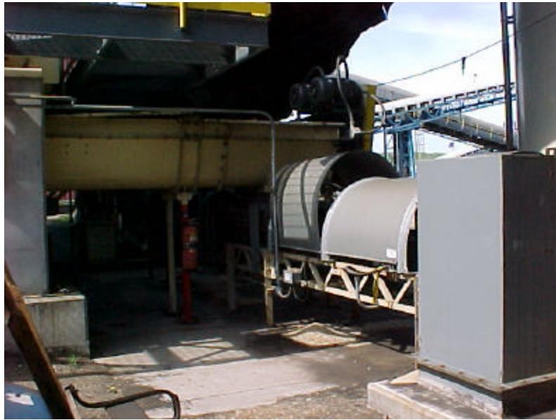
Figure 10. Weigh belt conveyor at Willow Island Generating Station
