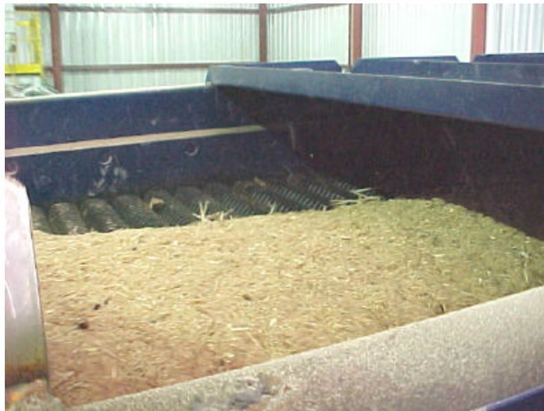
Figure 5. Screening sawdust at the Albright Generating Station
