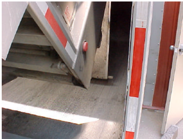
Figure 3. The lack of clearance between the walking floor sawdust receiver and the dump truck tailgate
