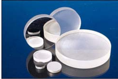
Figure 6. Photograph of optical flats, as used in optical biofouling tests.
