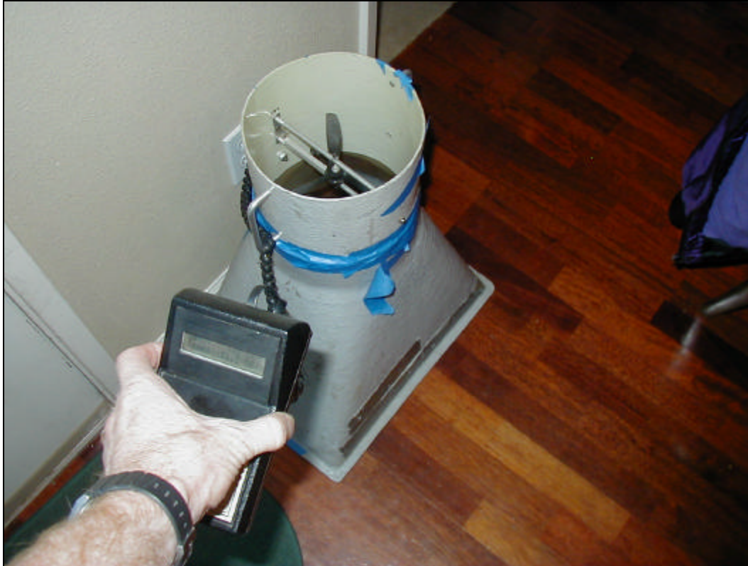
Figure 2-12. Measurement of supply register flow.
