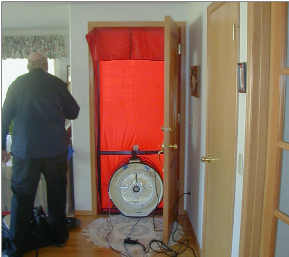
Figure 2-10. Blower door installed for Delta-Q test.
