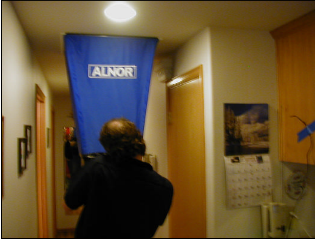
Figure 2-14. Measurement of return grille flow.
