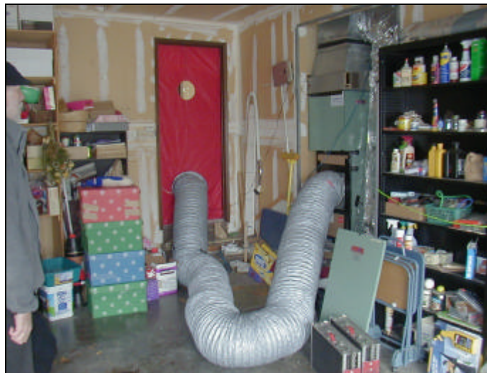
Figure 2-4. Calibrated fan attached to air handler within the conditioned space (left) and outside the conditioned space (right), such that air comes from house.
