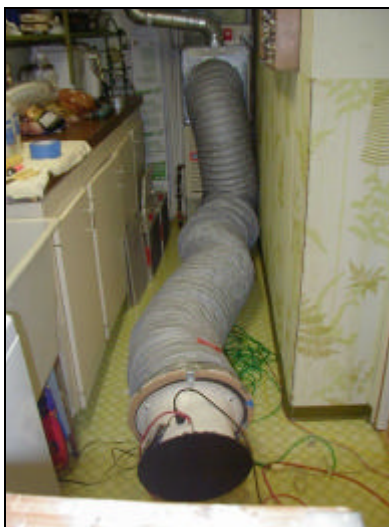
Figure 2-4. Calibrated fan attached to air handler within the conditioned space (left) and outside the conditioned space (right), such that air comes from house.
