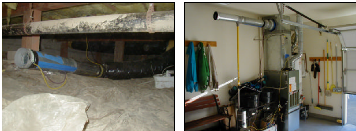
Figure 5-1. Examples of an added supply leak (left) and added return leak (right), measured with a calibrated flow station.
