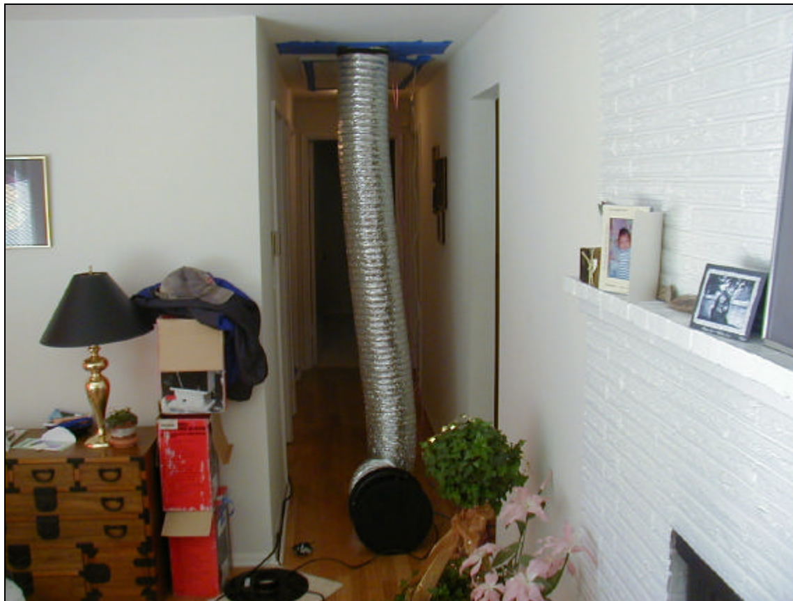
Figure 2-11. Calibrated fan attached to a return grille.
