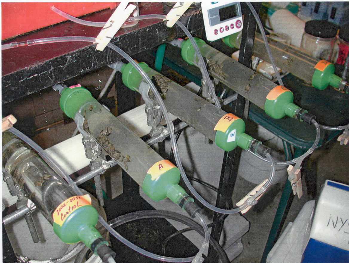
Fig. 1. Examples of the acrylic minipipes used in the tests described in this report. The pipe with clear water on left is an untreated control, whereas water in other pipes has a grayish color due to presence of suspended bacteria during treatment. Mussels are visible attached to walls of pipe.
