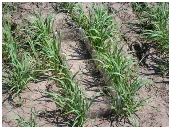
Figure 3. Nitrous oxide gas samples are collected using a vented chamber made of plexiglass. Without cover (left). With cover (right)
