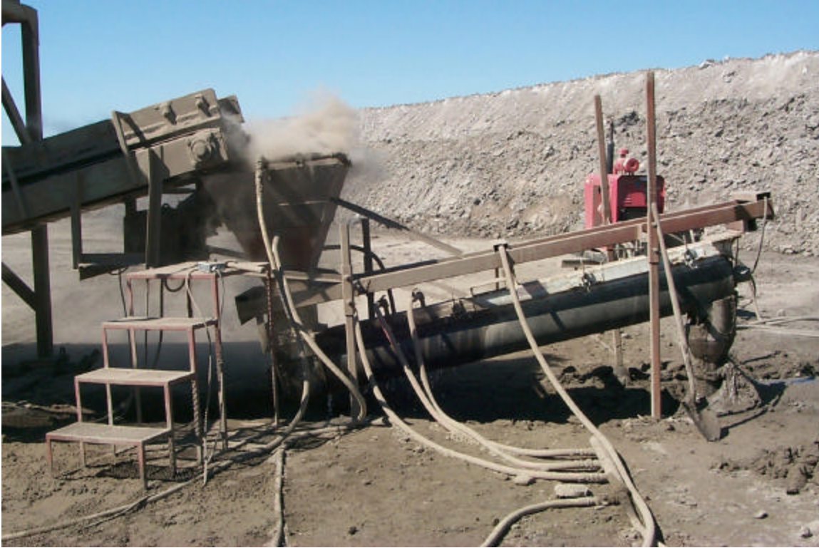
Figure 17. Backfilling operation using auger mixer.
