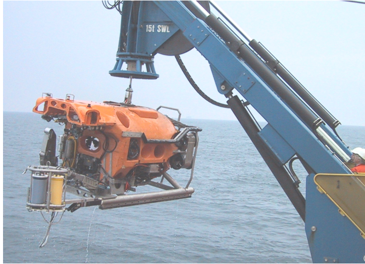
Figure 4: ROV and gravimeter during recovery.
