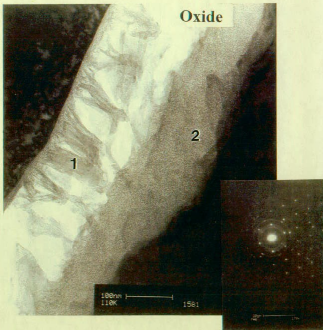
Figure 8. AEM bright field image showing cross-section of wide IGSCC crack away from carbides. Oxide corrosion product exhibits speckled and acicular morphologies. Electron diffraction pattern contains some NiO and unidentified textured phase. (Acid mildly oxidizing, 260°C, sensitized)
