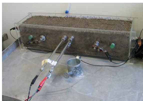
Figure 2- Soil test cell with three electrochemical electrodes and four electrodes for soil resistivity.
