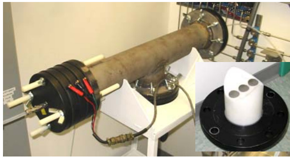
Figure 3 – Pipeline test cell with three flange electrodes and three disc electrodes (inset) in the side arm.
