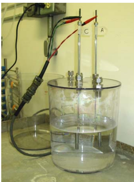
Figure 1- Test cell for aqueous solutions with three electrodes.
