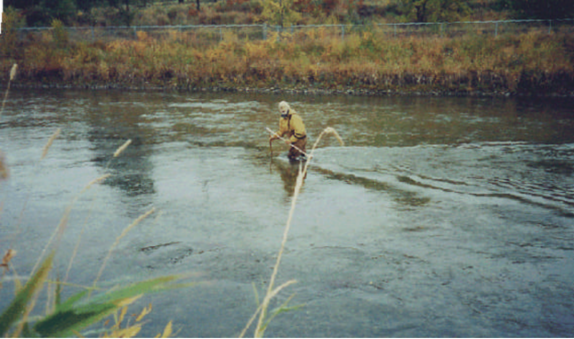
Figure 4-2: the average velocity was 1.4 m/s and average depth 0.55 m during spawning in reach G on October 18/01. The turbulence in the foreground is caused by spawning sockeye.
