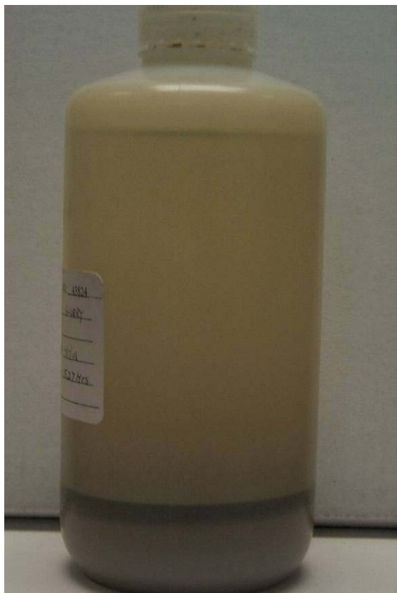
Figure 3.5-34: Fines in Endicott Wet FGD Slurry
