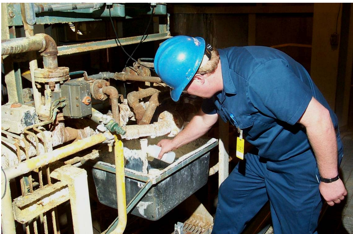
Figure 3.5-18: Wet FGD Slurry Sampling at Zimmer
