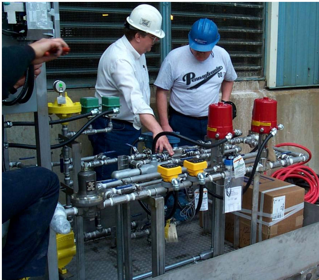
Figure 3.2-4: Reagent Injection Skid
