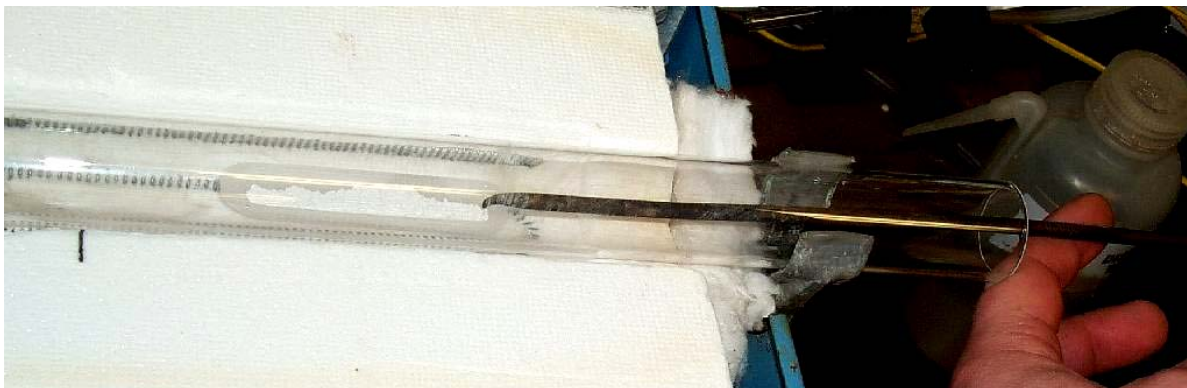
Figure 3.5-31: TDT, Inserting a Sample Boat into the Control Oven
