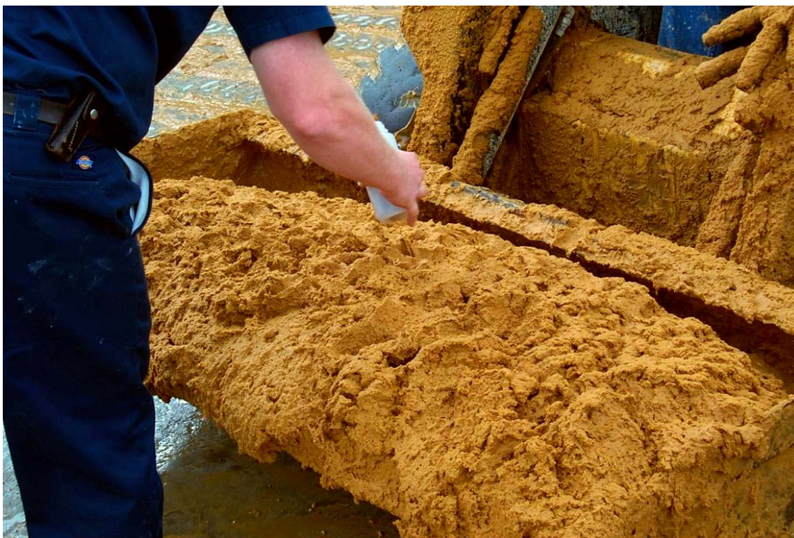
Figure 3.5-19: Wet FGD Slurry Fines from the Centrifuges at Zimmer
