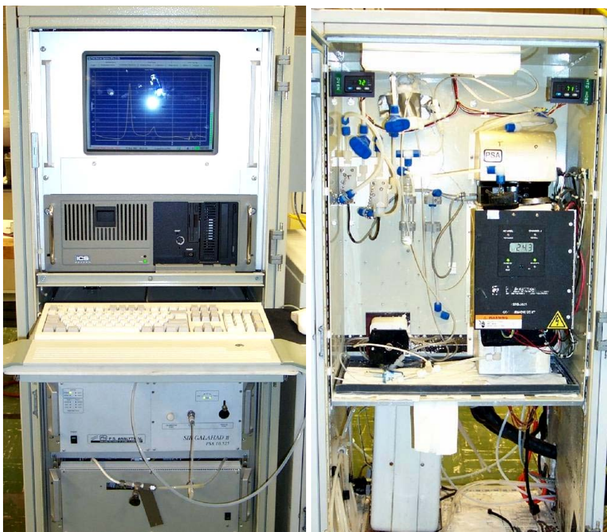
Figure 3.5-32: PSA Mercury Analyzer and Preconditioner
