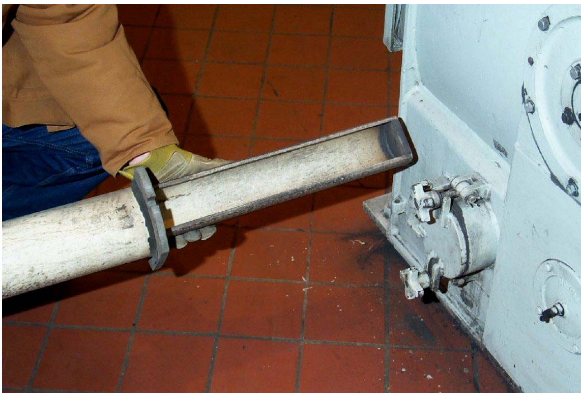
Figure 3.5-1: Endicott Coal Sampling Device and Pulverizer Feeder Sampling Port
