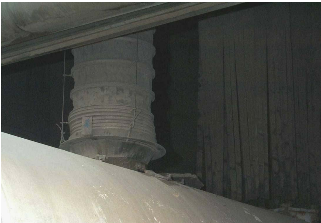
Figure 3.5-17: Ash from the South Ash Silo being Loaded into a Tanker at Zimmer
