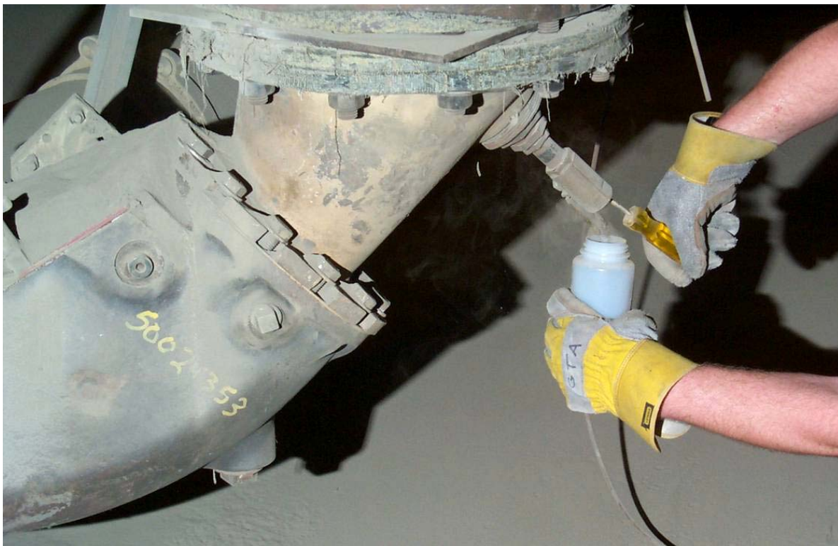
Figure 3.5-16: ESP Ash Sampling at Zimmer
