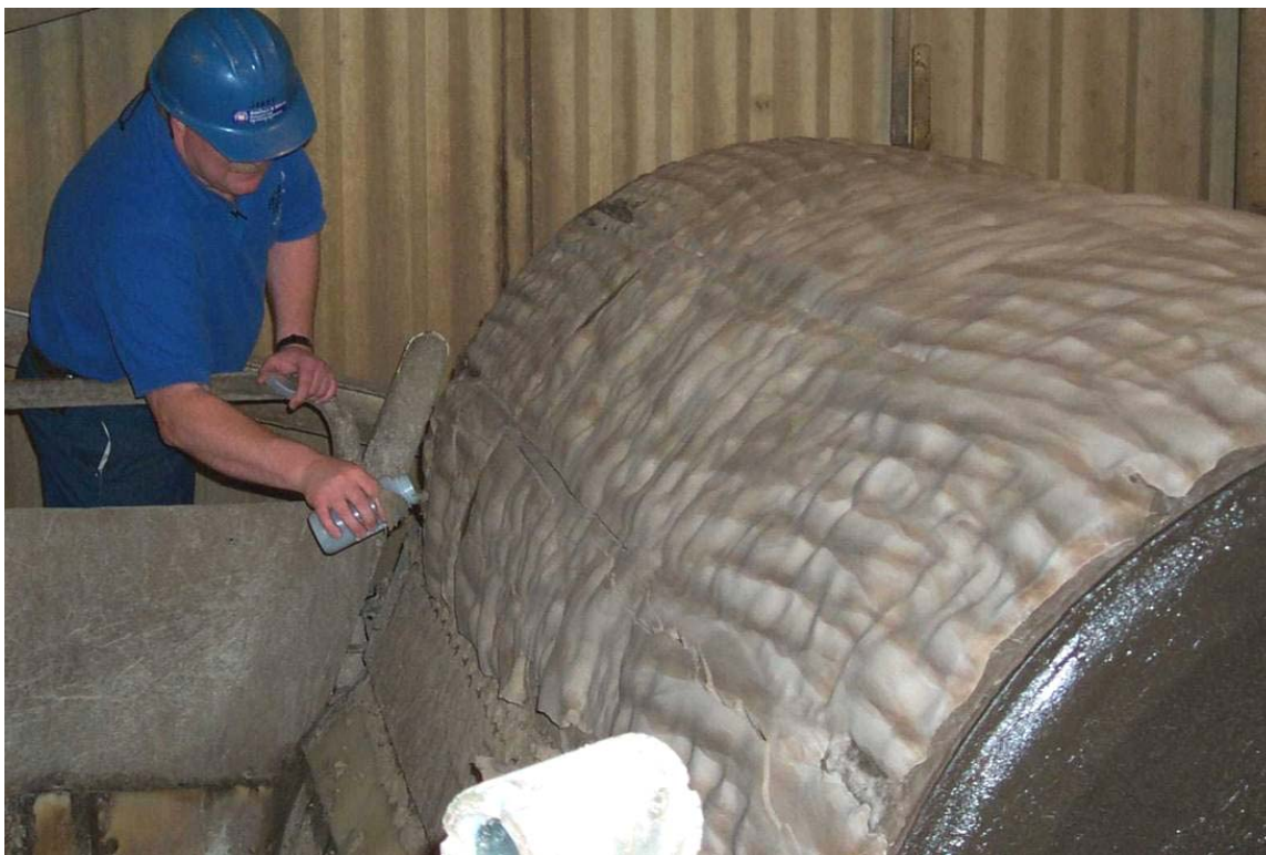
Figure 3.5-11: Gypsum Filter Drum at Endicott
