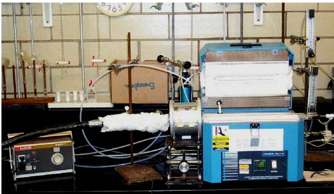
Figure 3.5-29: TDT Heated Hose, Pyrolyzer, Control Oven, Argon Flow Meters
