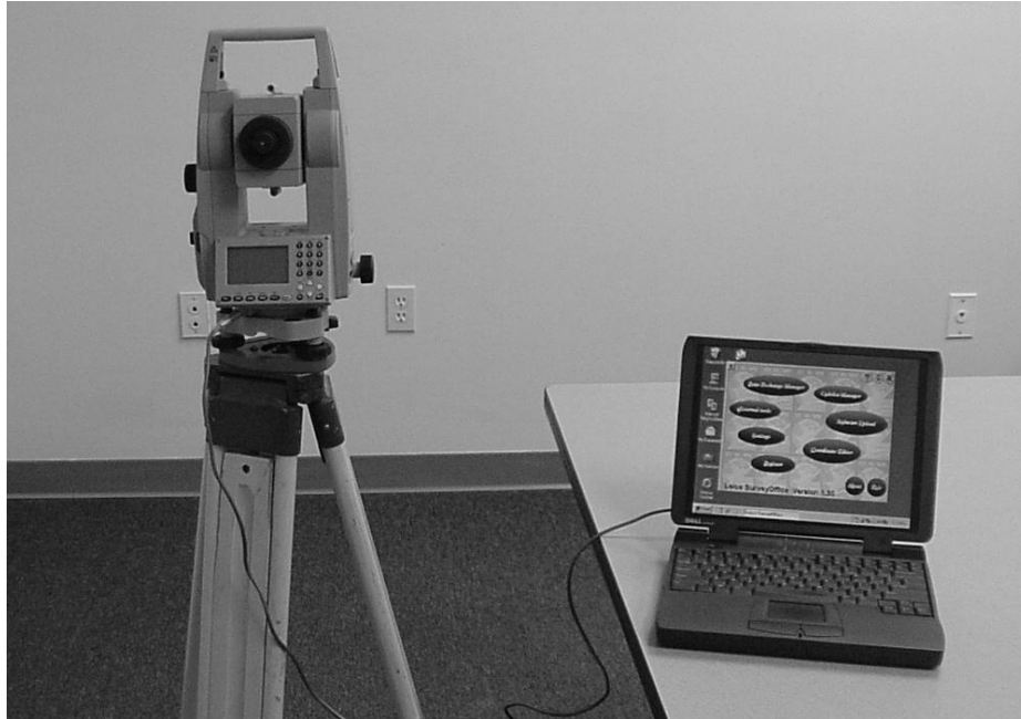
Figure 2.7. A Leica Total Station TCR 703, shown on tripod with APTI laptop computer connected for data download, was used to record the size of craters generated during field experiments.
