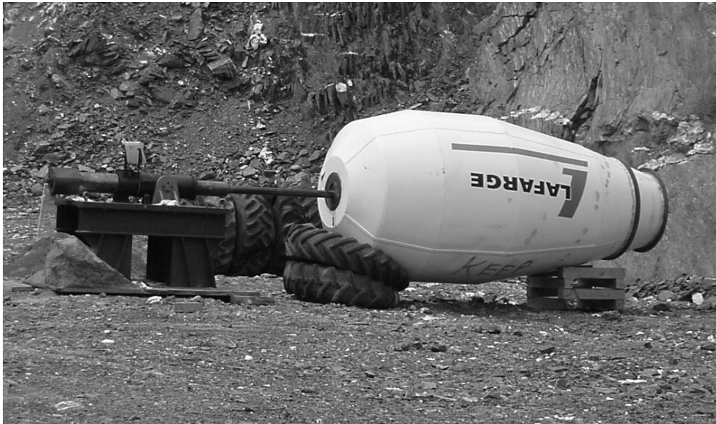
Figure 2.1. A 60 mm launcher was used for the Field Experiments with a drum muffler, shown here, following the failure of the tire muffler.
