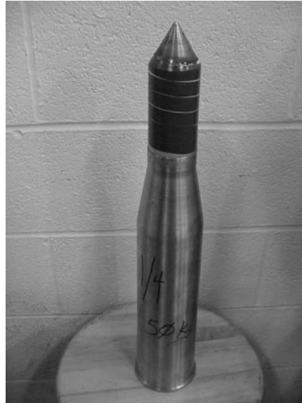
Figure 2.5. Steel encased rounds survived high acceleration forces during launch. Sketches of the rounds tested appear on the left, while a fully assembled 60 mm round, ready to fire, is shown on the right.
