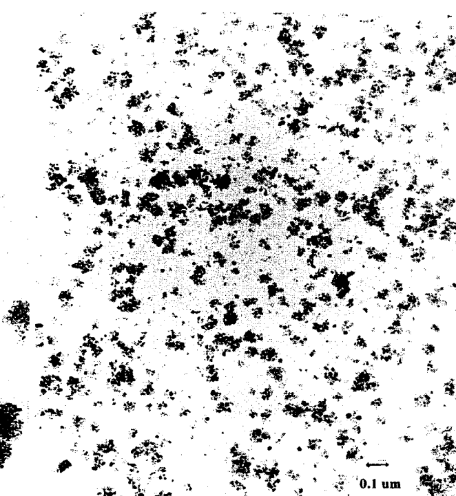
Figure 1b Sample 1b: PVA 250 11.97 % \text{Fe}_3\text{O}_4 100,000X
