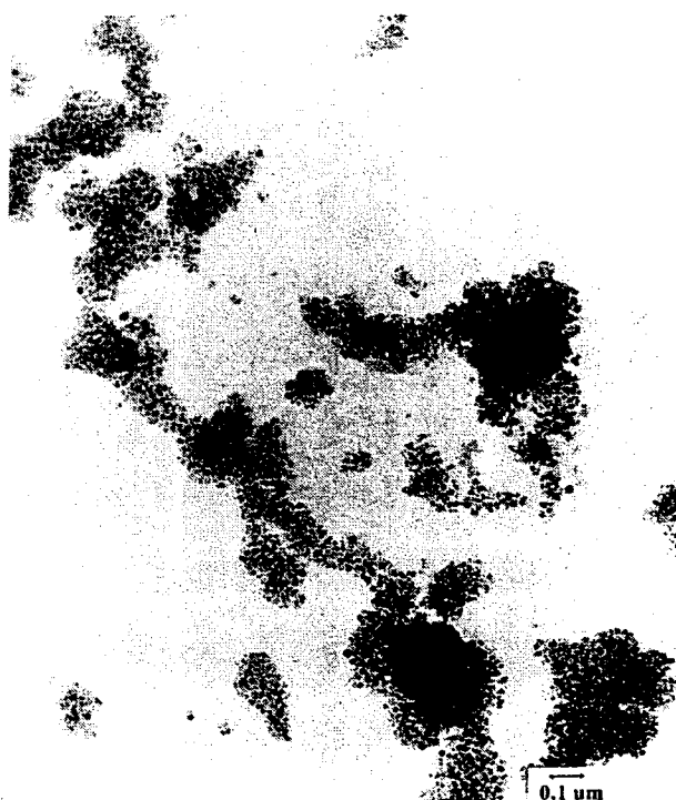
Figure 1a Sample: PVA 248 52.9% \text{Fe}_3\text{O}_4 100,000X
