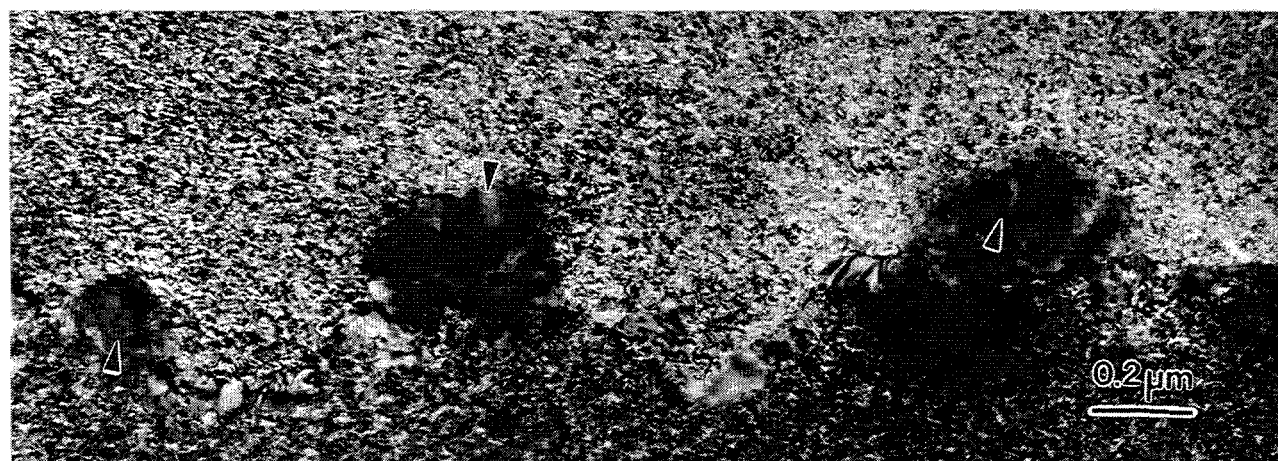
Figure 6. TEM micrograph of irradiated Heat A1 with three complex intergranular Cr-rich M_{23}C_6 / Ni,B-rich M_{23}X_6 agglomerated precipitates (arrowed).
