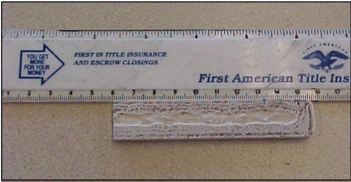
Figure 3: Compression Side of Test Bar Showing Sawn and Sanded Areas
