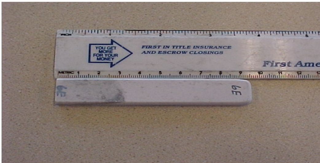
Figure 2. Tensile Side of the Molded Test Bar
