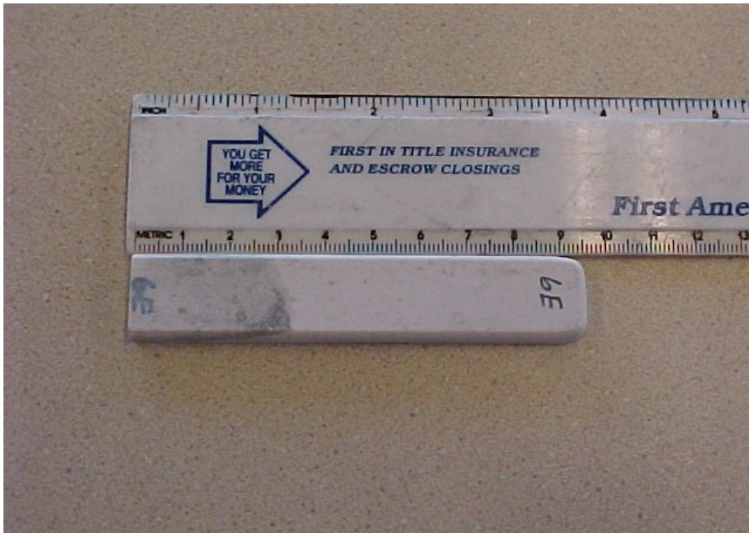
Figure-2. Tensile Side of the Molded Test Bar
