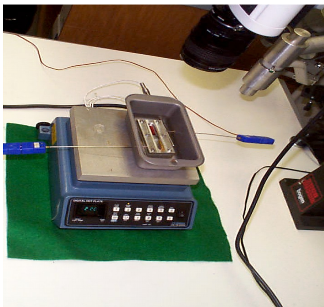
Figure 6: Water Bath and Hot Plate Setup
