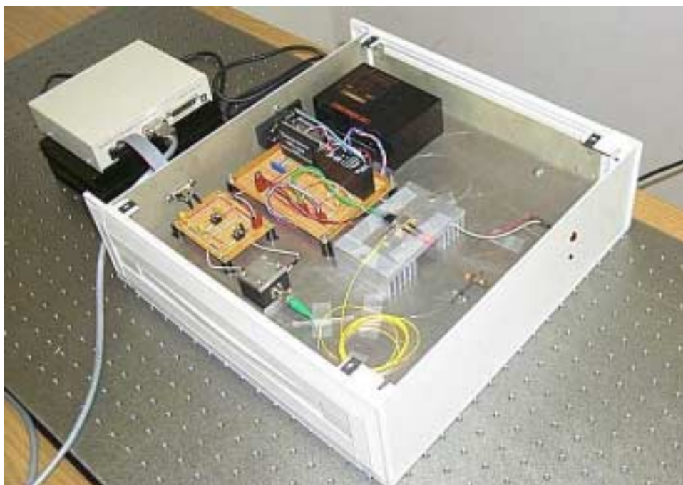
Figure 4.10. Singlemode fiber SCIIB sensor system, schematic (top) and photograph (bottom).
