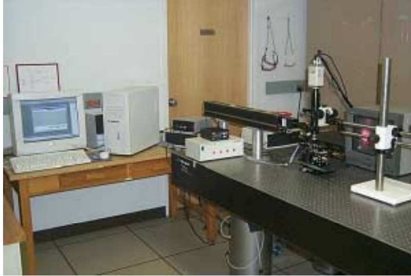
Figure 6.2. Automated SCIIB sensor fabrication system.
