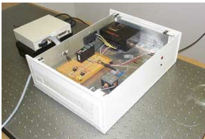
Figure 4.8. Multimode fiber SCIIB sensor system, schematic (top) and photograph (bottom).
