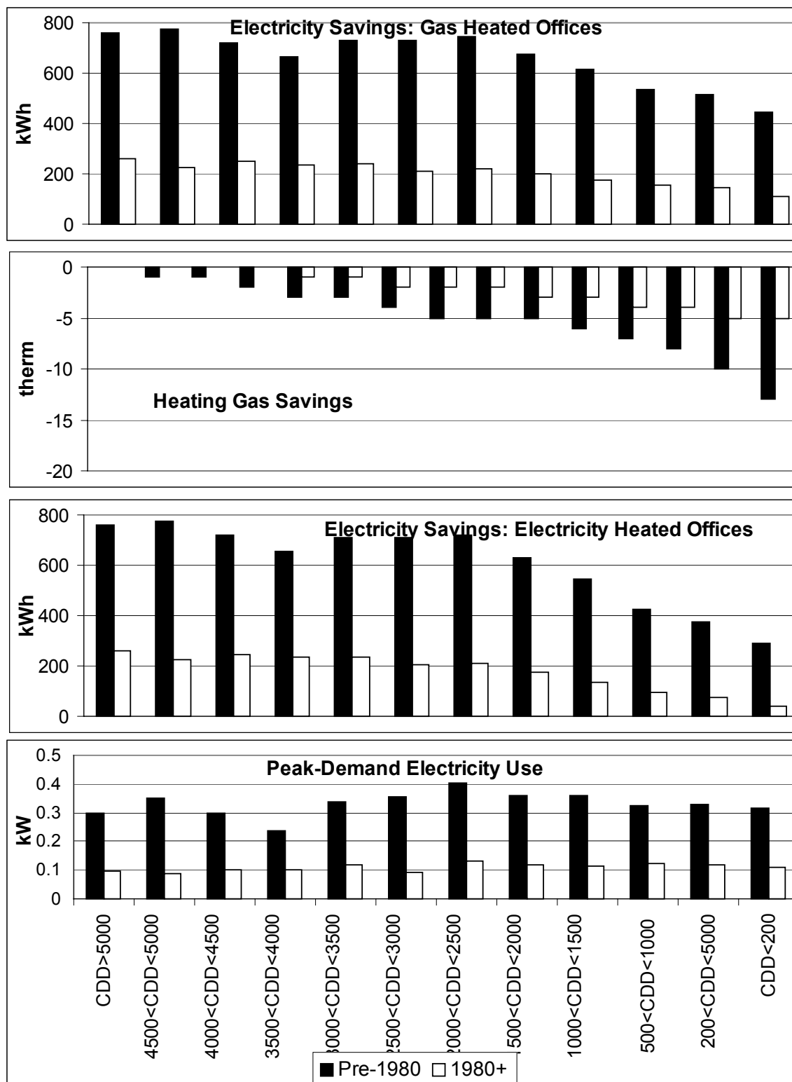
Figure 4b(ii). Office Buildings. Savings from Cool Roofs as a function of cooling-degree-days: Annual cooling-electricity savings and heating-gas savings for gas-heated houses, combined heating- and cooling-electricity savings for electrically heated houses, and peak-electricity demand savings. All estimates are normalized per 1000 ft 2 of roof area.
