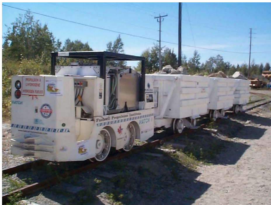
Figure 9. Fuelcell Locomotive Pulling 3 Fully Loaded 4 Ton Ore Cars
