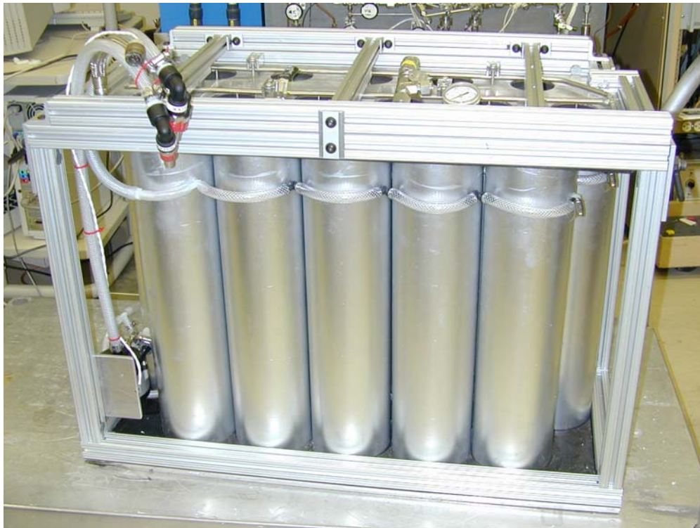
Figure 5. Metal-Hydride Storage Module
