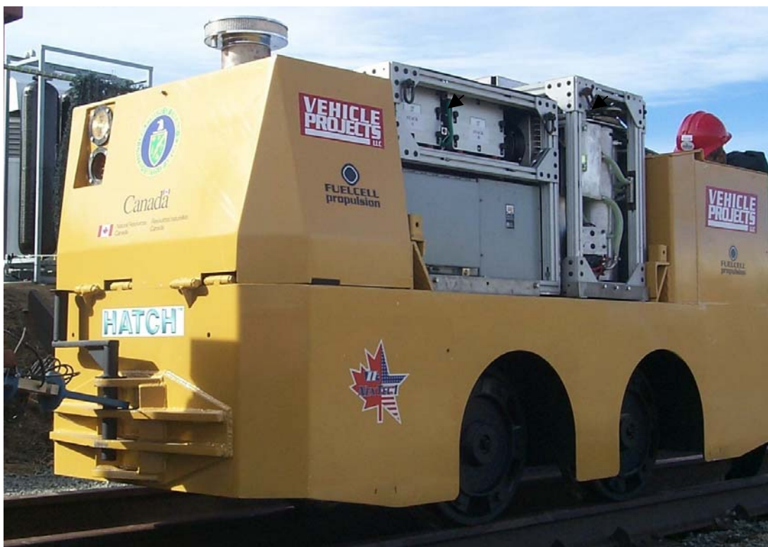
Figure 11. Final Version of Fuelcell Locomotive, Reno, NV
