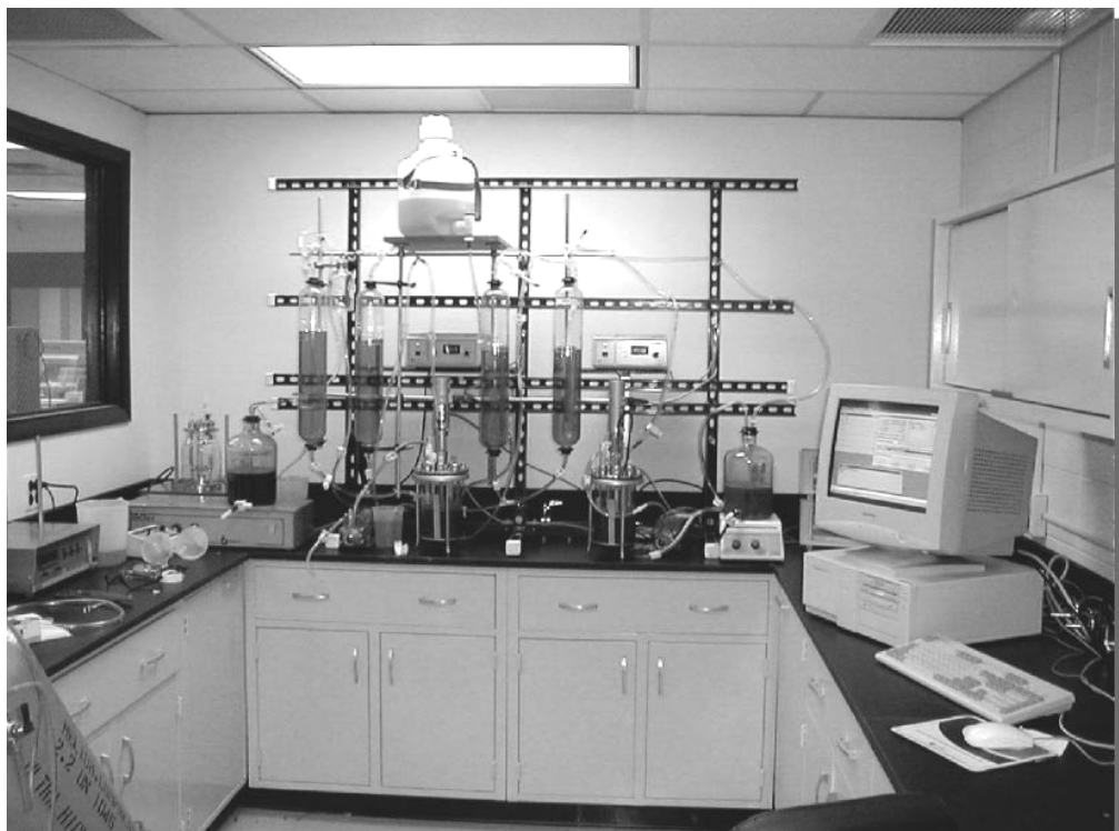
Figure 4.2 Two-phase anaerobic digester units processing manure & sewage sludge feedstocks
