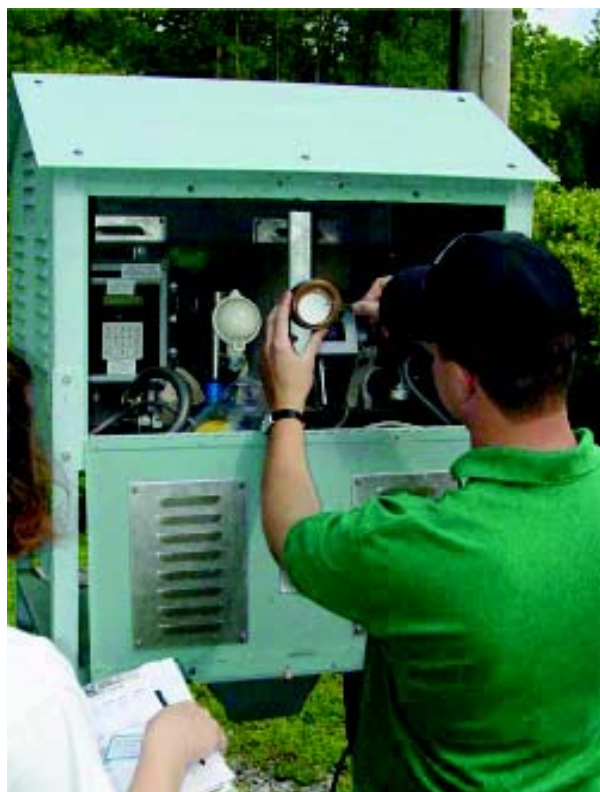
Changing an Air Filter at an Air Sampling Station
