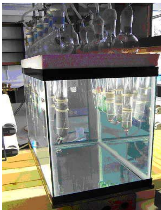
Fig. 3. General view of the photobioreactor with tubes coated with window mesh layer.
