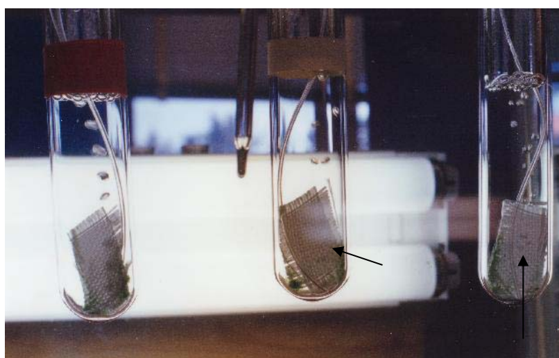
Fig.14. Coupons at the day after inoculation Black arrows point out that Omnisil coupon edges are colonized more significantly than central zones of these coupons.
