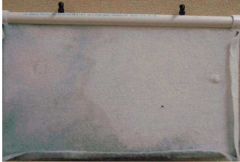
c. White polyester membrane after 72 hours' running in the CRF II test
