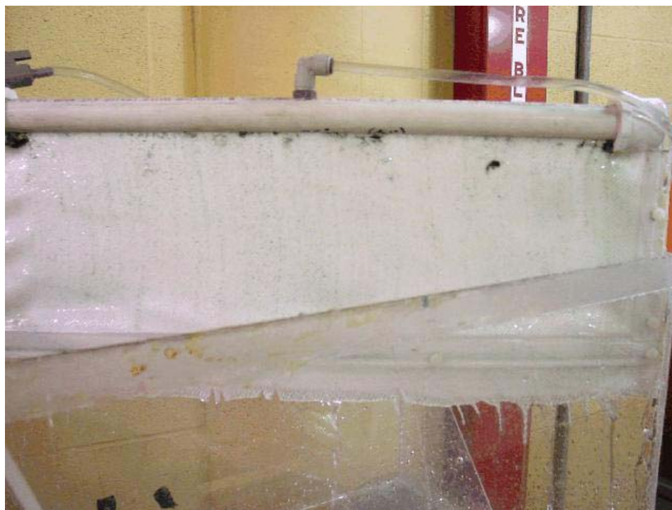
c. Screen loading effect after re-circulating 1.2. s.c.(2) for 60 mins
