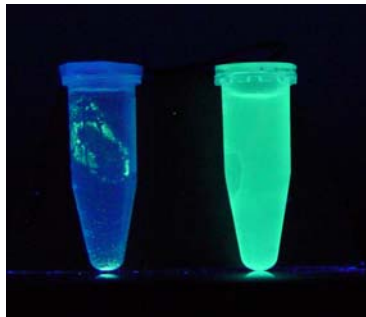
Figure. 1. left: composite of 3 and streptavidin-coated microspheres agglutinated at the bottom of the Eppendorf cap. The blue fluorescence stems from the Eppendorf cap. Right: control experiment in which 2 and streptavidin coated microspheres are mixed. No agglutination is observed.
